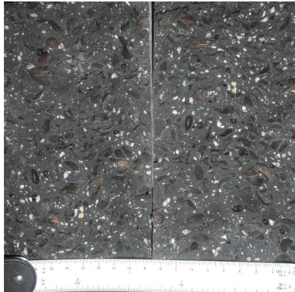
Figure 4.19: Bond failure of OPSGC
