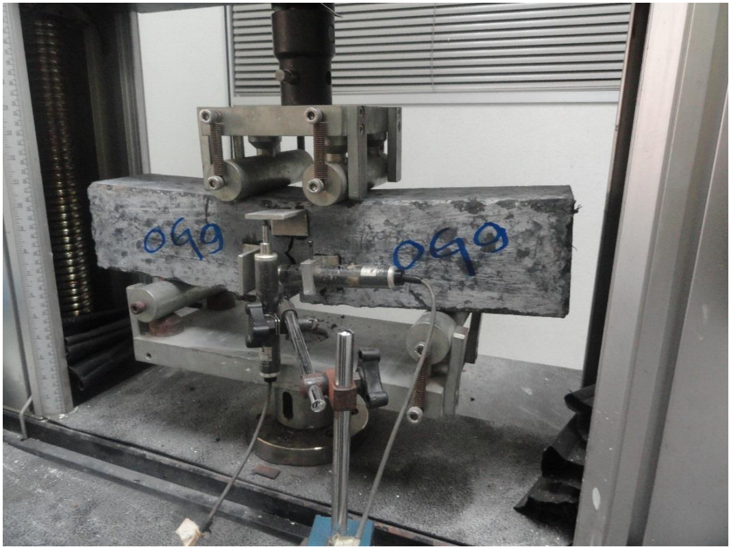
Figure 3.10: Fracture test (ASTM C1609/C1609M-12, 2012)
