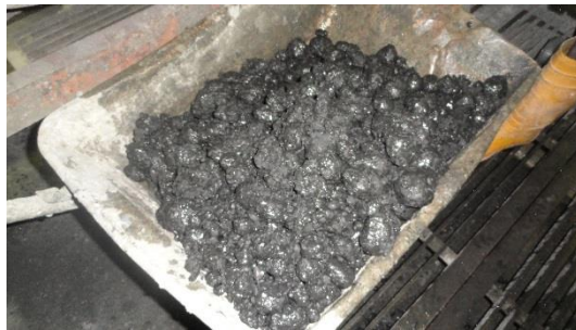
Photo B.14: OPSGC for casting
