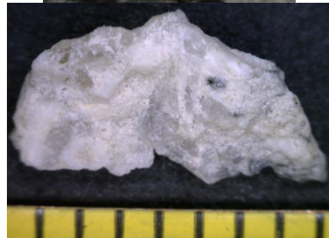
Figure 4.3: Particle shape of quarry dust (2.36 mm retained)
