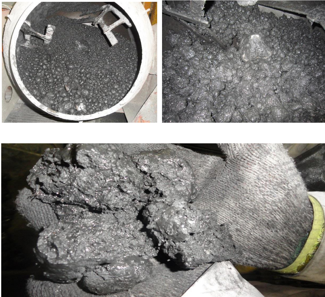
Figure 3.4: Casting of geopolymer fibre reinforced concrete
