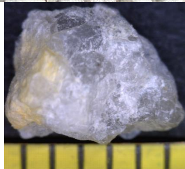
Figure 4.2: Particle shape of manufactured sand (2.36 mm retained)
