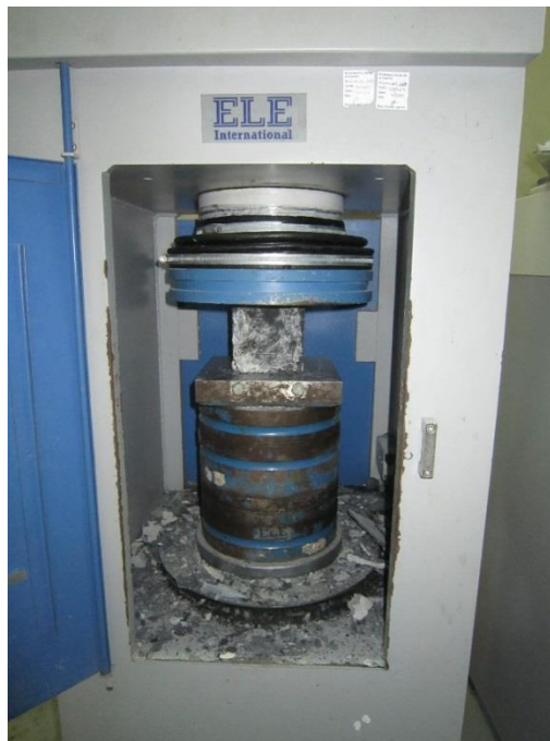
Figure 3.6: ELE testing machine of capacity 2000 kN
