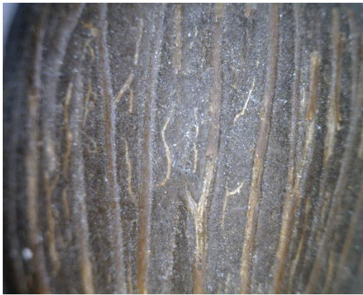
Photo B.9: Outer surface of OPS
