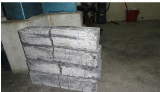
Photo B.11: Broken prisms after flexure test
