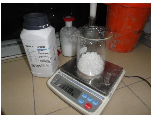
Photo B.5: Preparation of NaOH solution for trial
