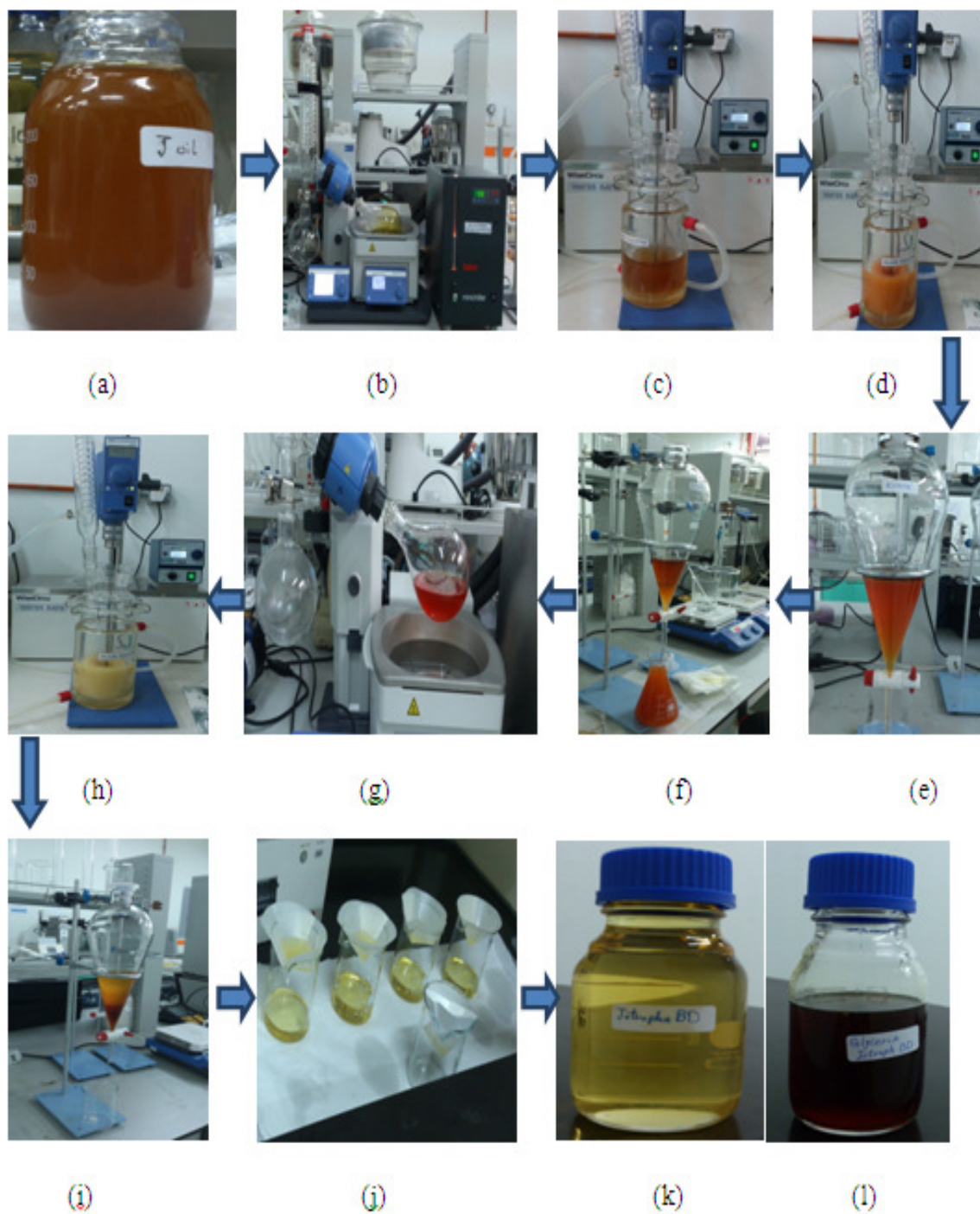
Figure 3.3: Biodiesel Production Process (a) Crude Oil (b) Remove Moisture (c) & (d) Esterification (e & f) Removal of Impurities (g) Removal of Methanol and Water (h) Transesterification (i) Settling (j) Filtering (k & l) Biodiesel & Glycerol respectively
