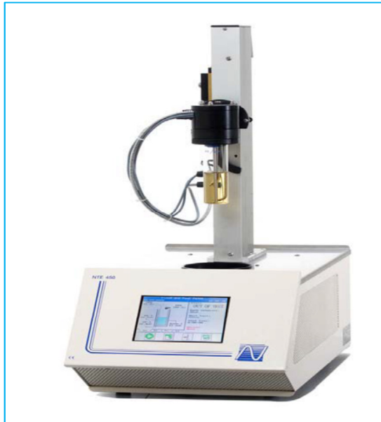
Figure 3.8: NTE 450 CP and PP Tester (Norma Lab, France)
