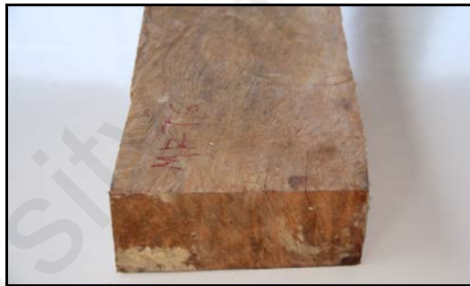
Figure 3.2. Original specimen from sawmill of 50 mm by 175 mm cross section of 2130 mm length plank.
