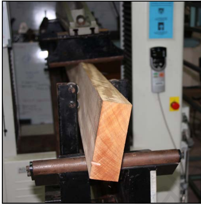
Figure 4.10. Twisted specimen resulted in buckling during test.
