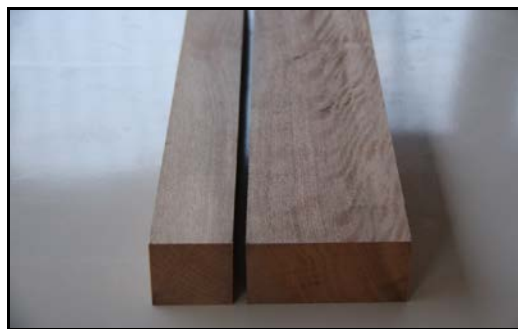
Figure 3.3. Specimen size of 50 mm x 50 mm x 750 mm and 50 mm x 100 mm x 1900 mm cut from the original plank.
