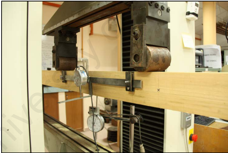
Figure 3.7. Experimental setup for structural size bending test.
