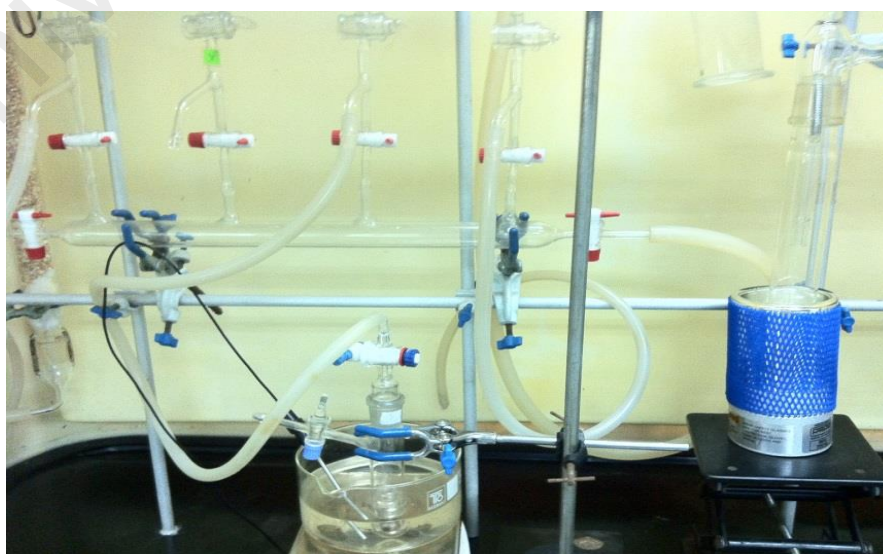
Figure 3.1: Drying of ionic liquid by Schenk line.
