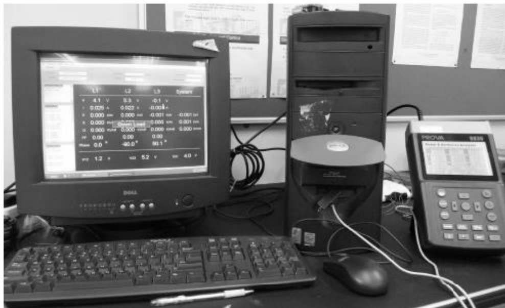
Power Analyzer is connected to the PC to save all data collected
