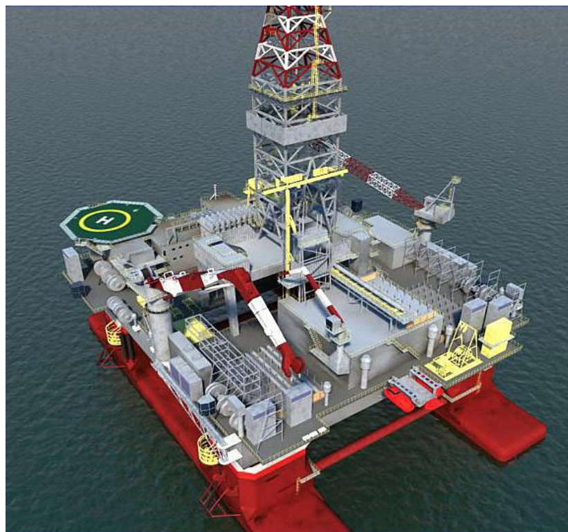
Figure 2.4: Semi-submersible offshore platform (Blushoes, 2010)
