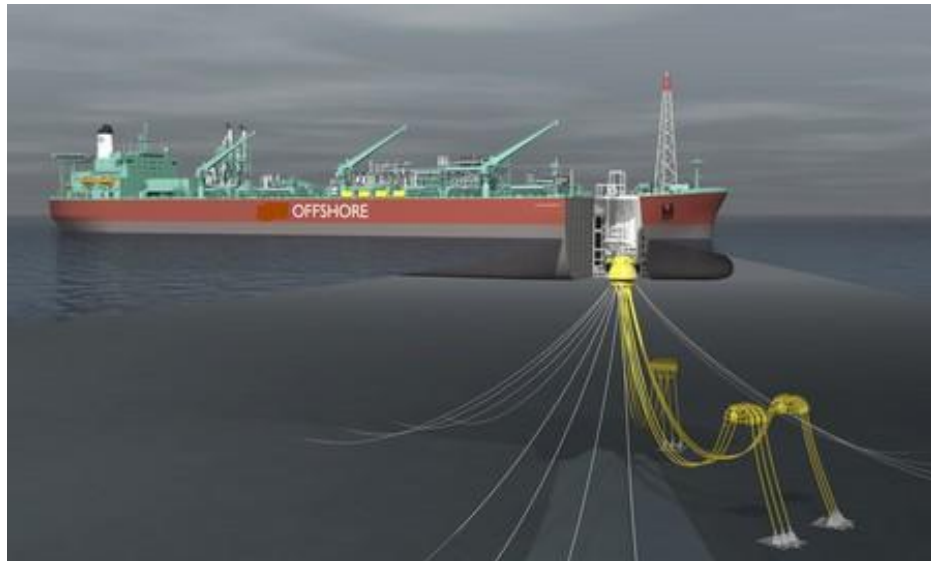
Figure 2.6: Floating production storage and offloading (FPSO) (MacGregor et al., 2000)
