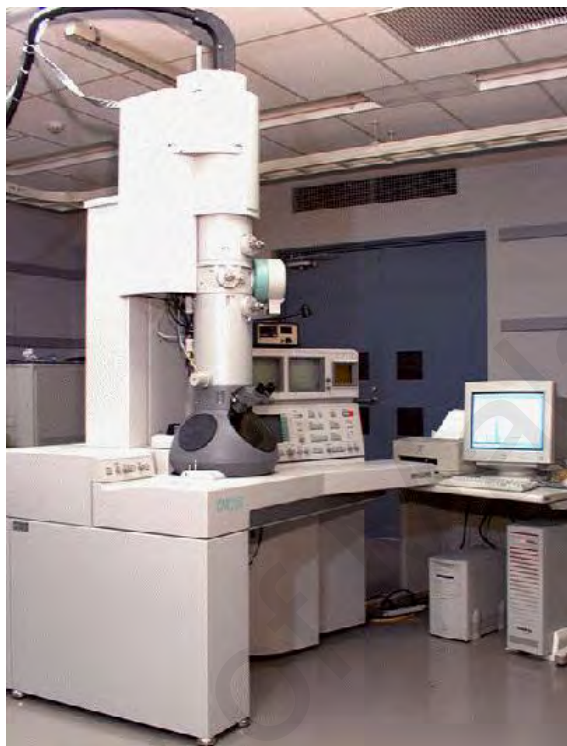
Figure 3.4: TEM microscope unit (Philips CM200) photograph
