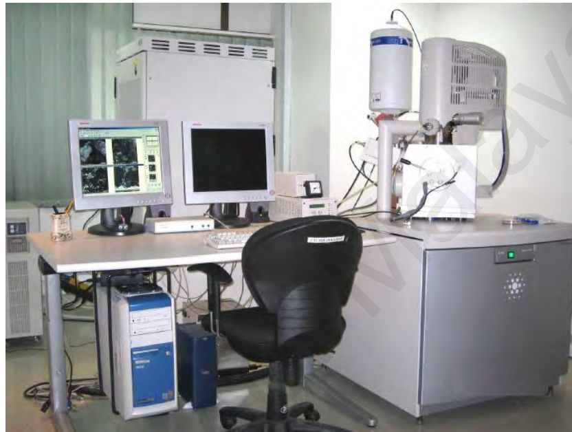
Figure 3.3: A set up of the FEI Quanta 200F FESEM equipped with EDX
