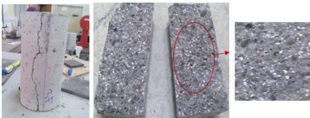
Figure 4.12: Failure pattern after splitting tensile strength test
