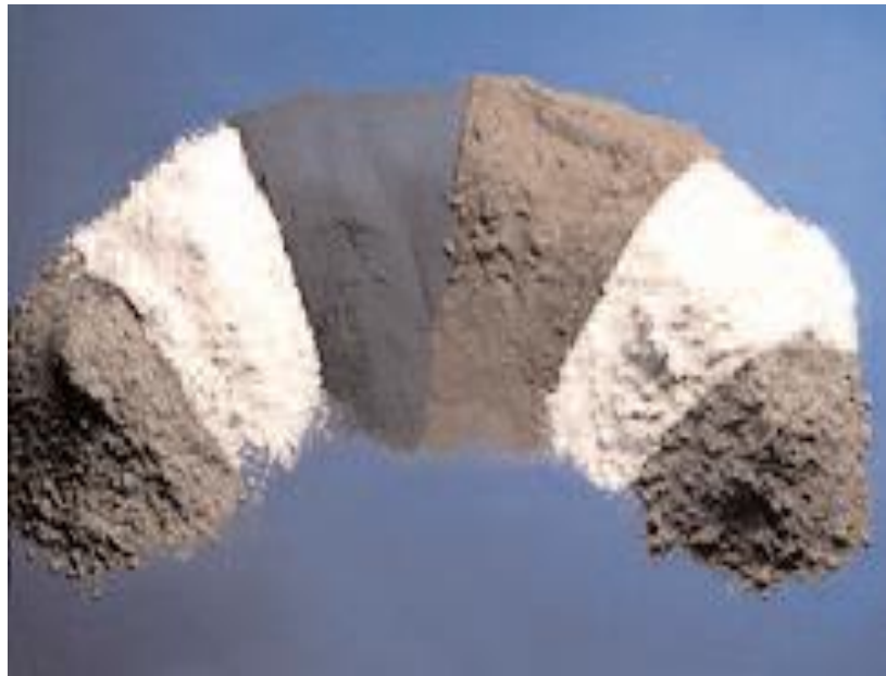
Figure 2.1: Cementitious materials. From left to right, fly ash (Class C), metakaolin (calcined clay), silica fume, fly ash (Class F), slag, and calcined shale
