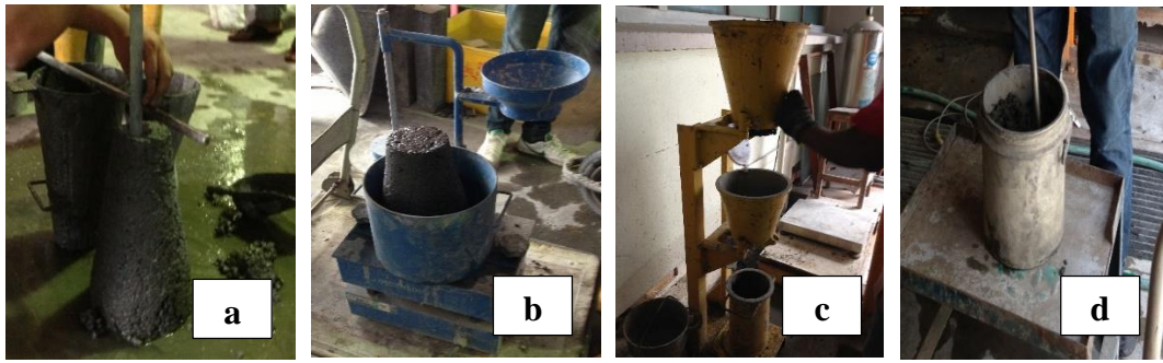
Figure 3.3: Test apparatus: (a) slump test, (b) vebe test, (c) compaction factor test and (d) wet density
