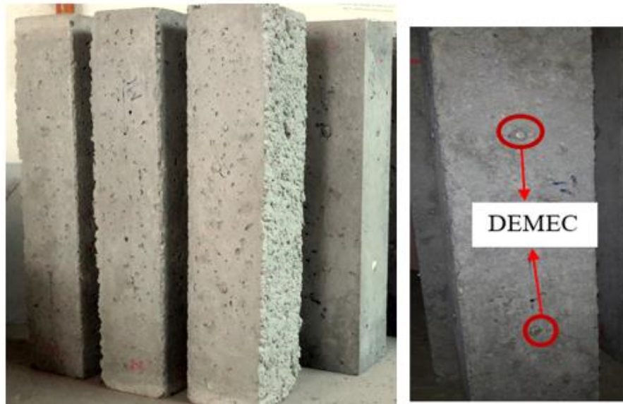
Figure 3.5: Drying samples with DEMEC studs.
