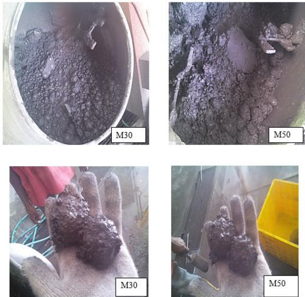
Figure 4.17: Mix M30 and M50 in concrete mixer machine at lower super-plasticizer content
