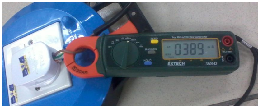
Figure 3.10 Voltage and current measurement on a single phase motor
