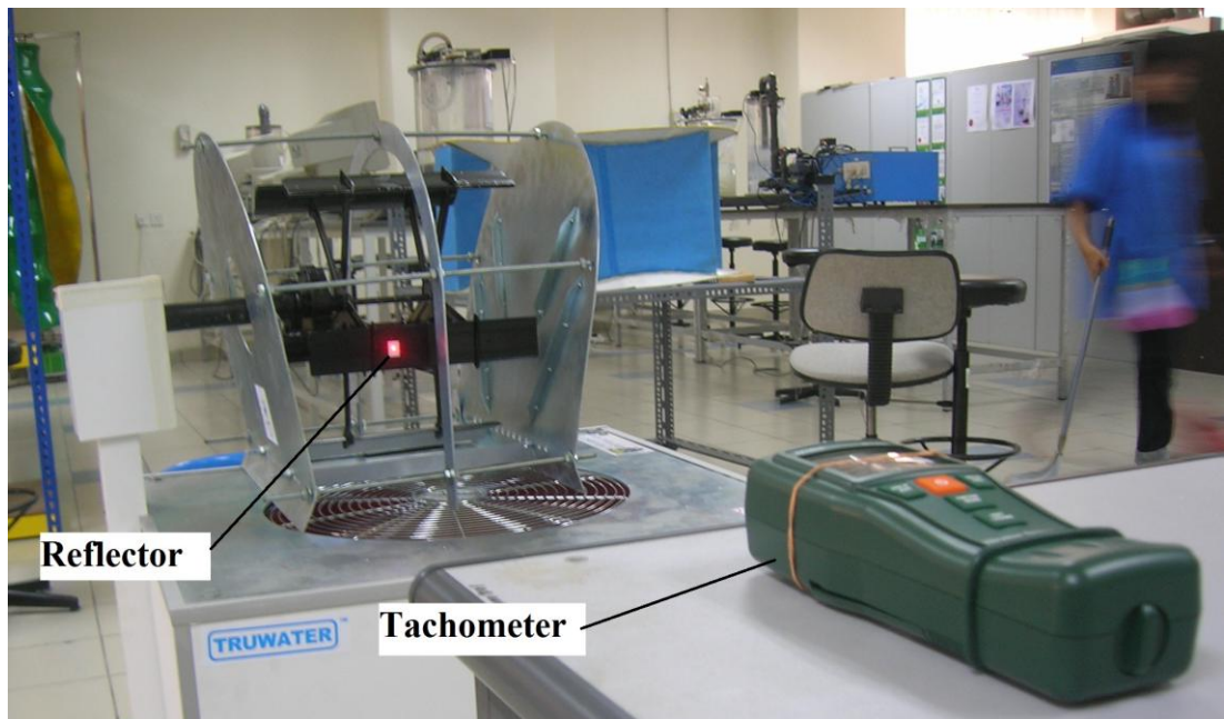
Figure 3.13 Wind turbine rotational speed measurement at laboratory testing. The tachometer is pointed to the turbine blade.
