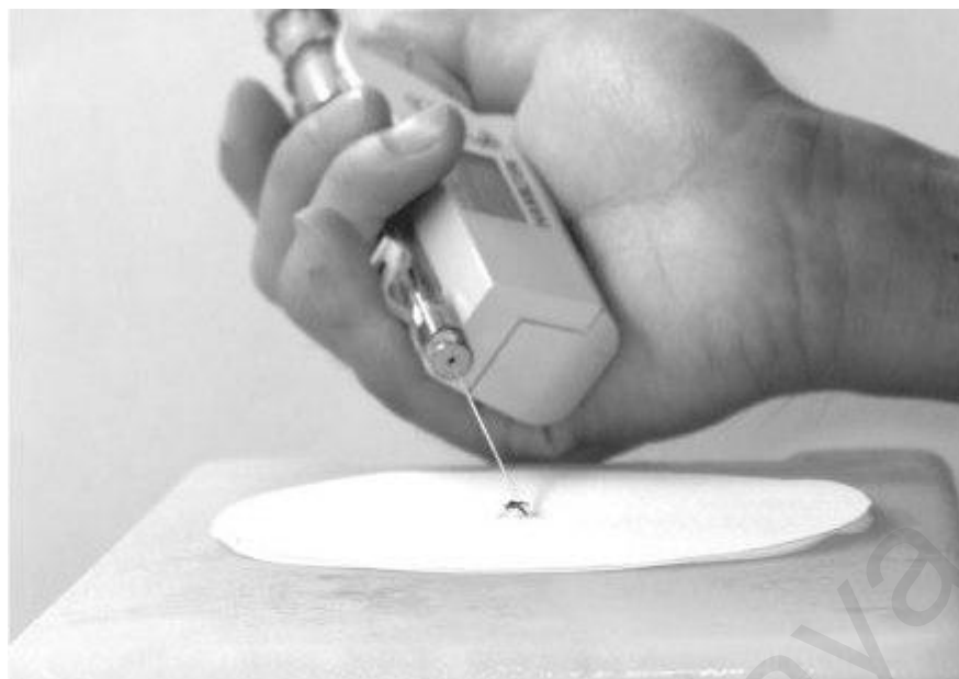
Figure 5.10: WHO standard protocols of topical application female mosquito using digital syringe (WHO, 1995).
