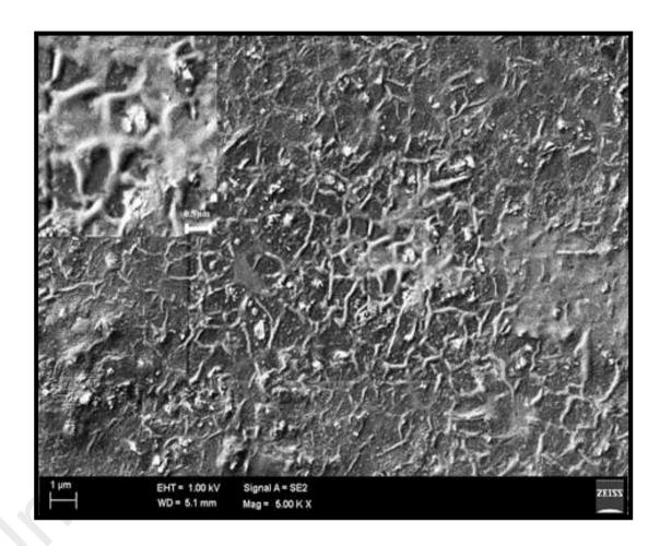
Figure 4.1: FESEM image of Bi<sub>2</sub>Te<sub>3</sub> composite film. Insert shows a high
