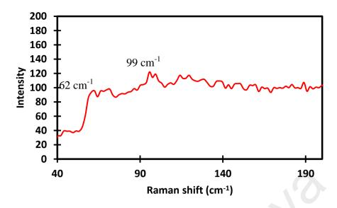
Figure 4.3: Raman spectrum of the free standing Bi<sub>2</sub>Te<sub>3</sub>-PVA film.
