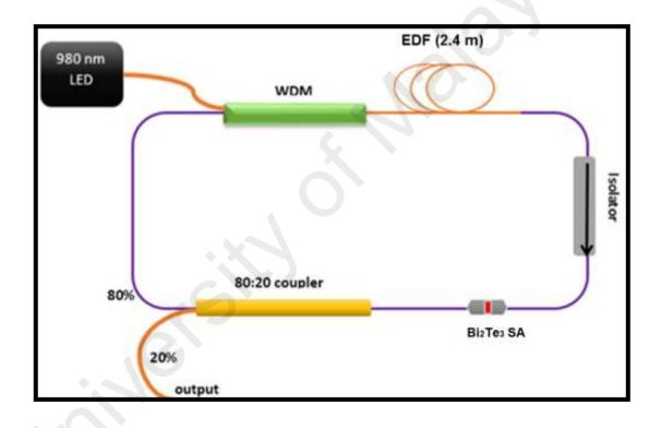
Figure 4.5: Configuration of the Q-switched EDFL with Bi<sub>2</sub>Te<sub>3</sub> PVA film.
