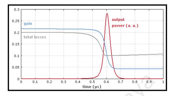
Figure 2.5: The evolution of gain and losses in passive Q-switching technique.
