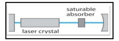
Figure 2.4: Basic structure of passive Q-switch laser cavity (Paschotta, 2008).
