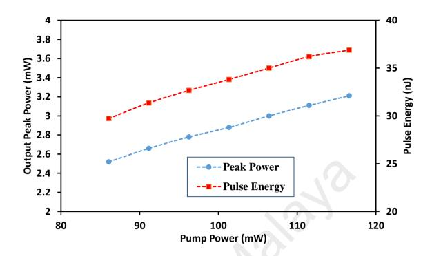
Figure 3.10: Pulse energy and peak output power as a function of pump power.
