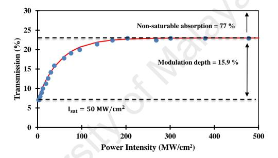
Figure 3.4: Nonlinear absorption characteristic for the Bi<sub>2</sub>Se<sub>3</sub>-PVA film.
