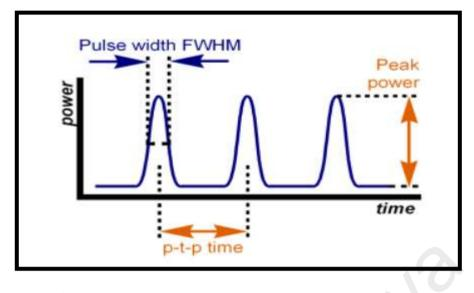
Figure 2.6: The important pulsed laser parameters
