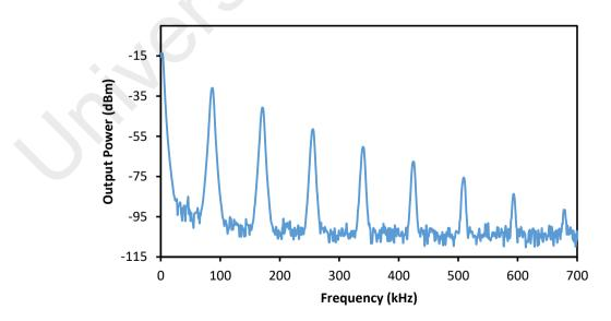
Figure 3.11: RF spectrum for the EDFL with Bi<sub>2</sub>Se<sub>3</sub> SA at 116.6 mW pump power.
