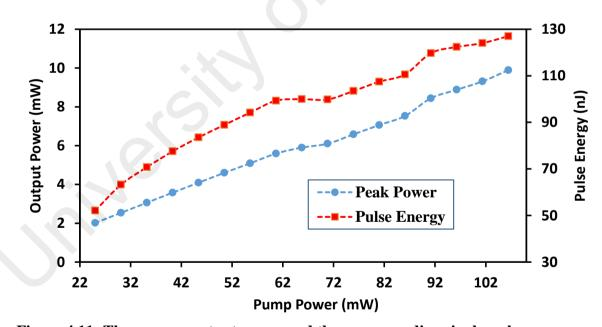
Figure 4.11: The average output power and the corresponding single-pulse energy against pump power.
