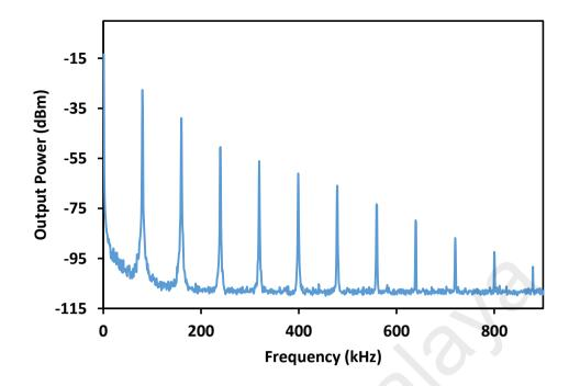
Figure 4.9: RF spectrum for the EDFL with Bi<sub>2</sub>Te<sub>3</sub> film-based SA at 106.4 mW pump power.
