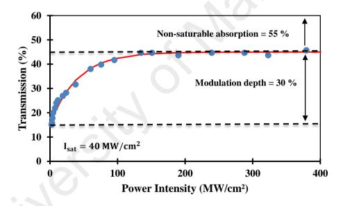
Figure 4.4: Nonlinear absorption profile for the Bi<sub>2</sub>Te<sub>3</sub> PVA film.
