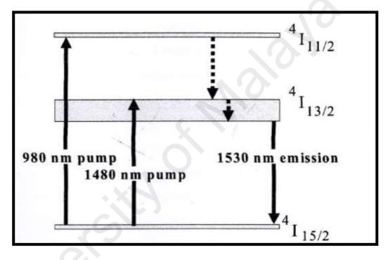
Figure 2.3: Illustration of energy level diagram of  $\text{Er}^{3+}$  ions in silica fibers (Zhu et al., 2015).
