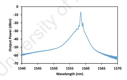
Figure 4.6: Emission spectrum of the EDFL with Bi<sub>2</sub>Te<sub>3</sub> film-based SA at 106.4 mW pump power.
