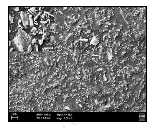
Figure 3.1: FESEM image of the Bi<sub>2</sub>Se<sub>3</sub> composite film. Insert shows the image with higher magnification.
