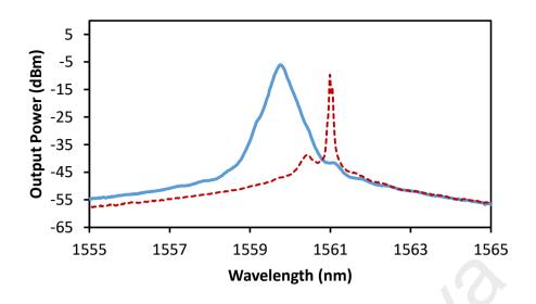
Figure 3.6: Output spectrum of the EDFL configured with and without Bi<sub>2</sub>Se<sub>3</sub> based SA at pump power of 116.6 mW.
