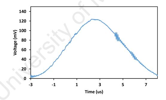
Figure 3.8: A single pulse envelop for the EDFL with Bi<sub>2</sub>Se<sub>3</sub> SA at 116.6 mW pump power showing a pulse width of 5.11 μs.
