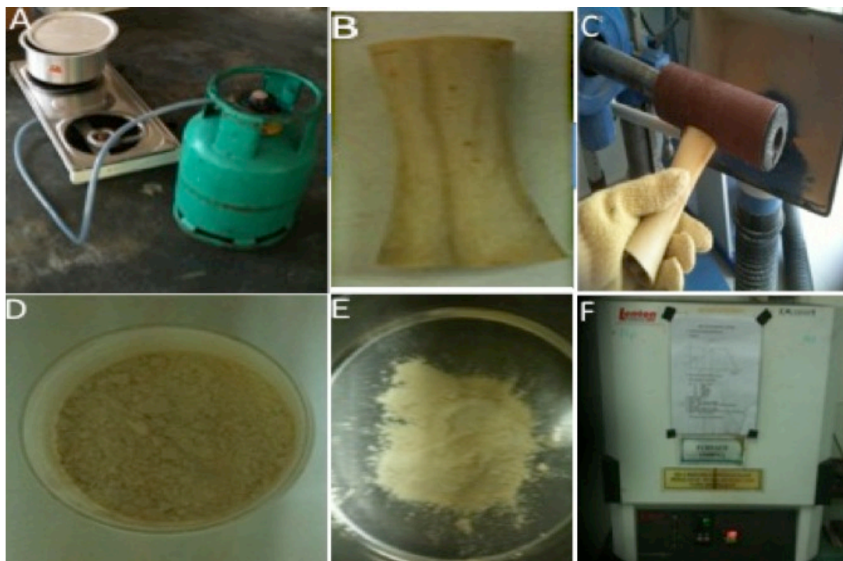
Figure 3.4: Bovine Hydroxyapatite production. A: Raw bovine bones are defatted; B: Dried Defatted Bone; C: Dried bone is then ground into powder; D: Bone powder is obtained; E: Powder is then sieved between 25\text{-}40\ \mu\text{m} ; F: Sieved powder is then heated to 1100^{\circ}\text{C} in a furnace.
