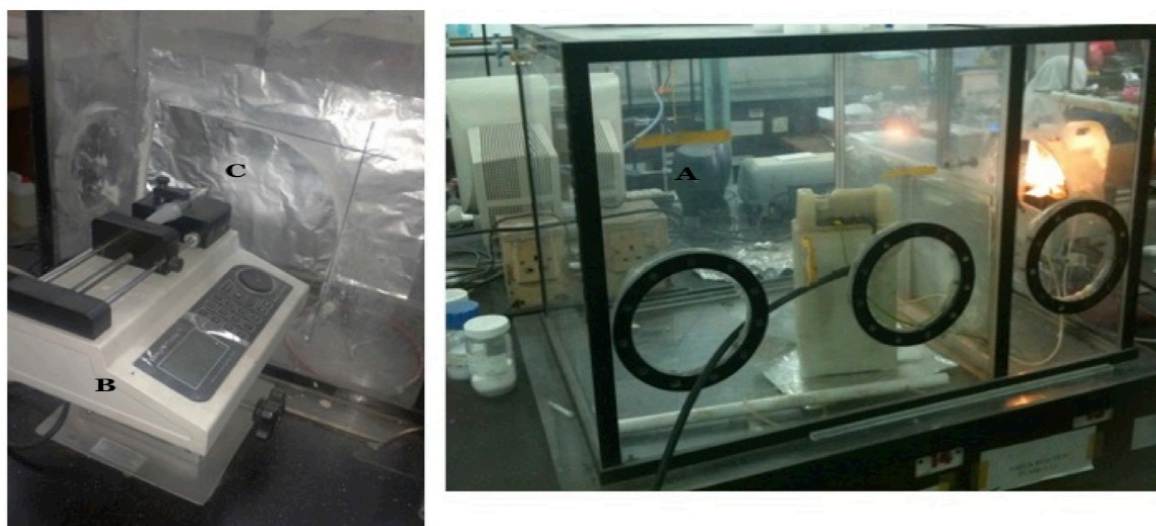
Figure 3.5: (i) Electrospinning machine setup which includes A: Box with minimal airflow for electrospun sheet; B: Syringe Pump; C: Aluminium sheet onto which electrospun scaffold was formed.
