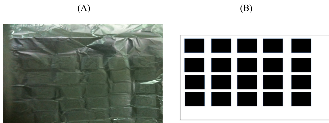
Figure 3.6: (A) Glass cover slips stuck on the aluminium sheet to prevent sticking of the electrospun sheet on the aluminium sheet. (B) Schematic representation of cover slips on aluminium sheet.
