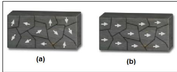
Fig 2.6. (a) Domains before magnetization. (b) Domain after magnetization (Reproduced from http://hyperphysics.phy-astr.gsu.edu/ ).
