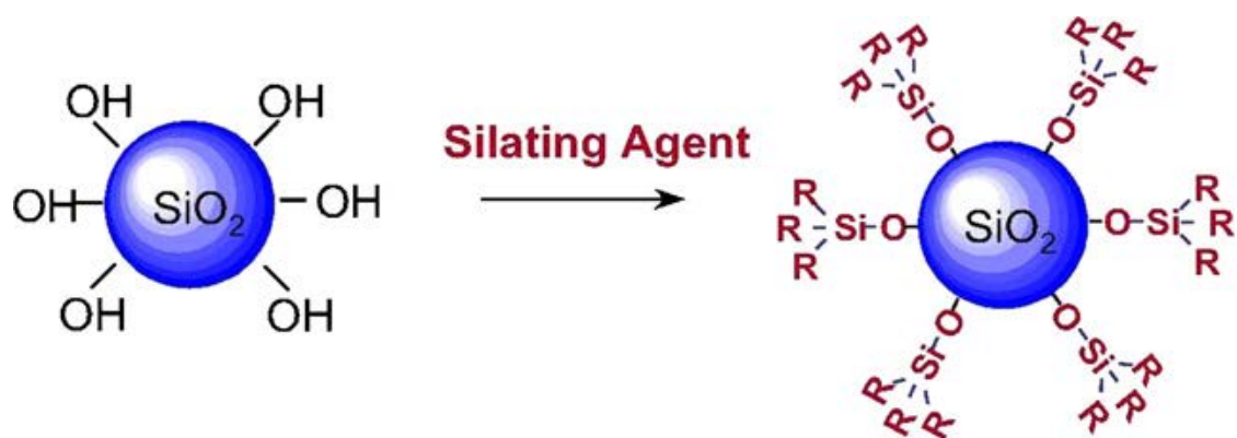
Figure 2.4: Effect of silylation on silica network in silica gel (Dorcheh and Abbasi, 2008b)
