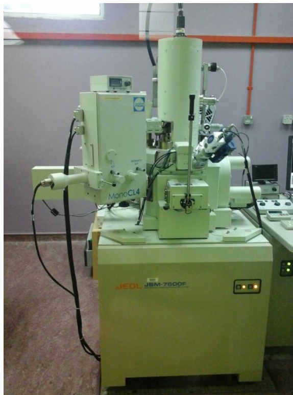
Field Emission Scanning Electron Microscope (FESEM) Physics Department University of Malaya
