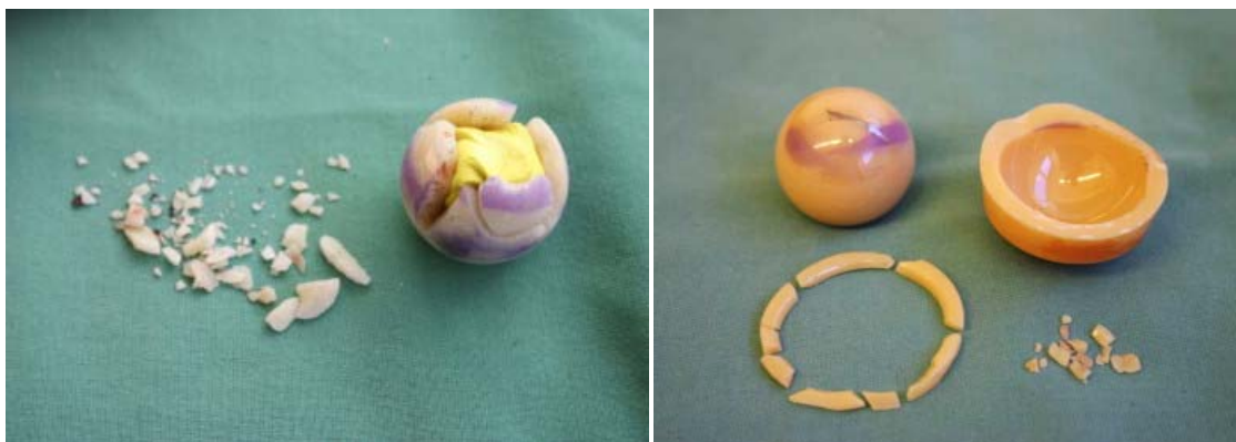
Figure 2.7: Fractures in a ceramic ball and acetabulum cup (Jenabzadeh et al., 2012)
