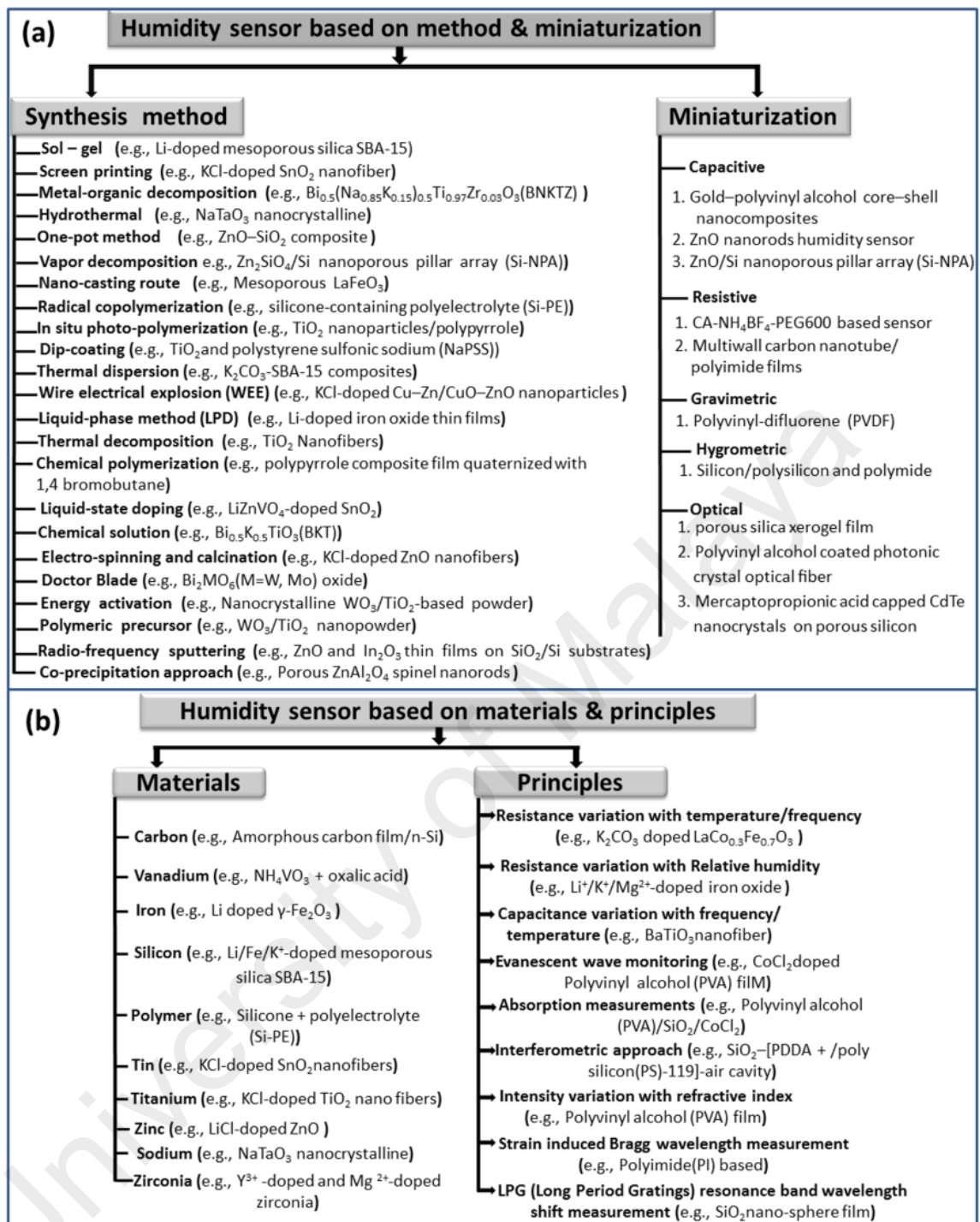
Figure 2.1: Humidity sensors based on (a) synthesis method and miniaturization, (b) Humidity sensors based on materials and principle.
