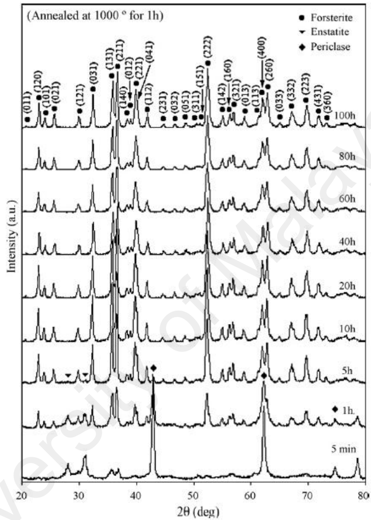
Figure 3.1: Phase purity result of forsterite powder milled at various durations and subsequently heated at 1000 °C for 1 hour (Tavangarian & Emadi, 2009).
