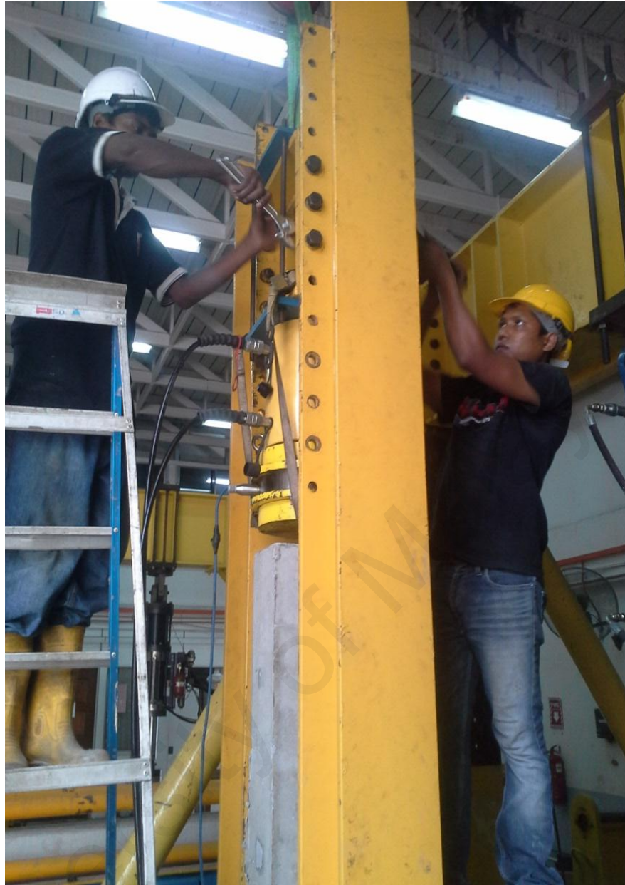
Figure 3.17: Fixing and dismantling of beam-column specimen
