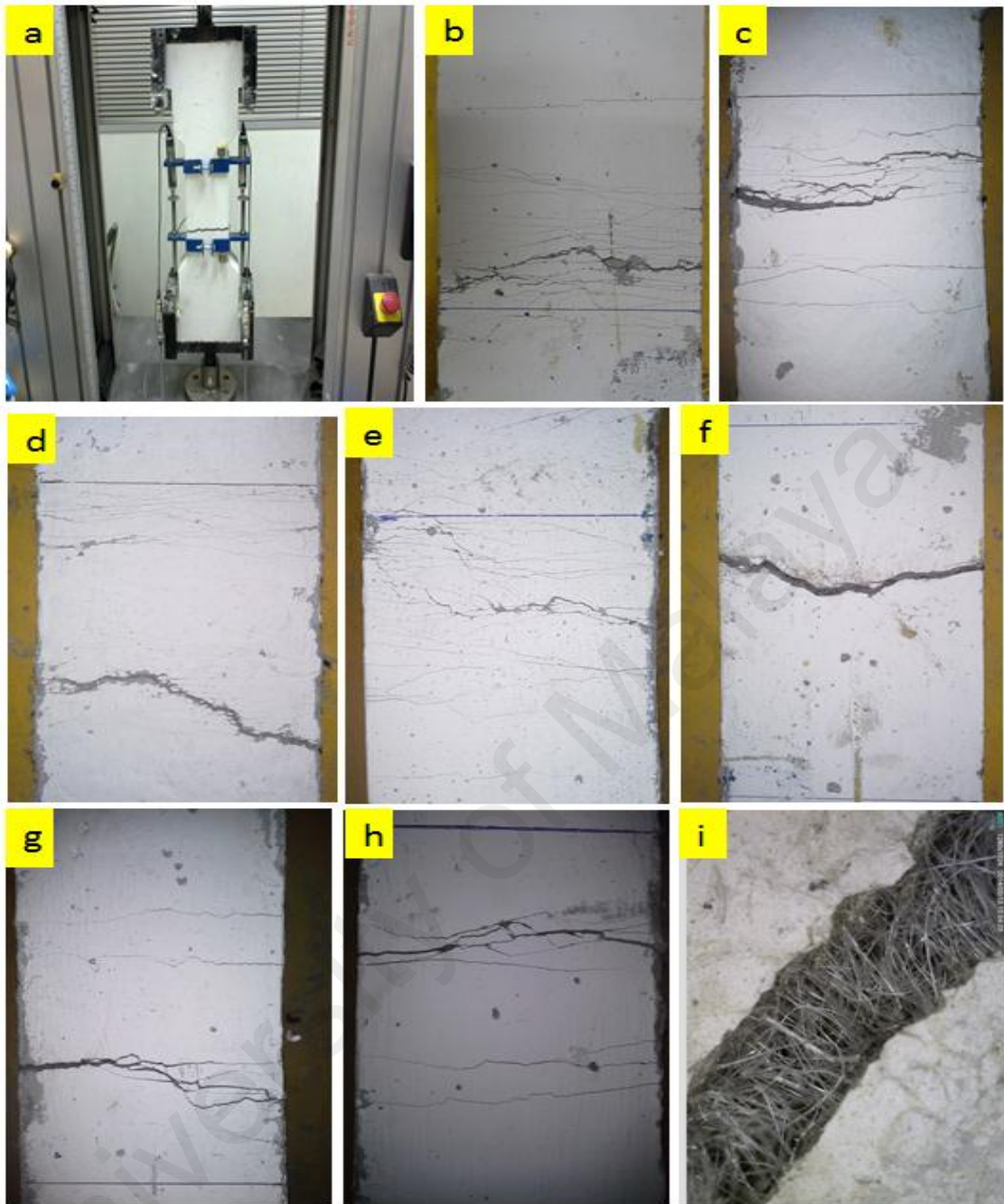
Figure 4.25: (a) I-shaped sample under tensile loading. Crack propagation in: (b) TPE 2 (c) TPE 4 (d) TPE 5 (e) TPE 7 (f) TPVA 2 (g) TPVA 7 (h) TPVA 8 (i) Crack bridging in I-shaped sample
