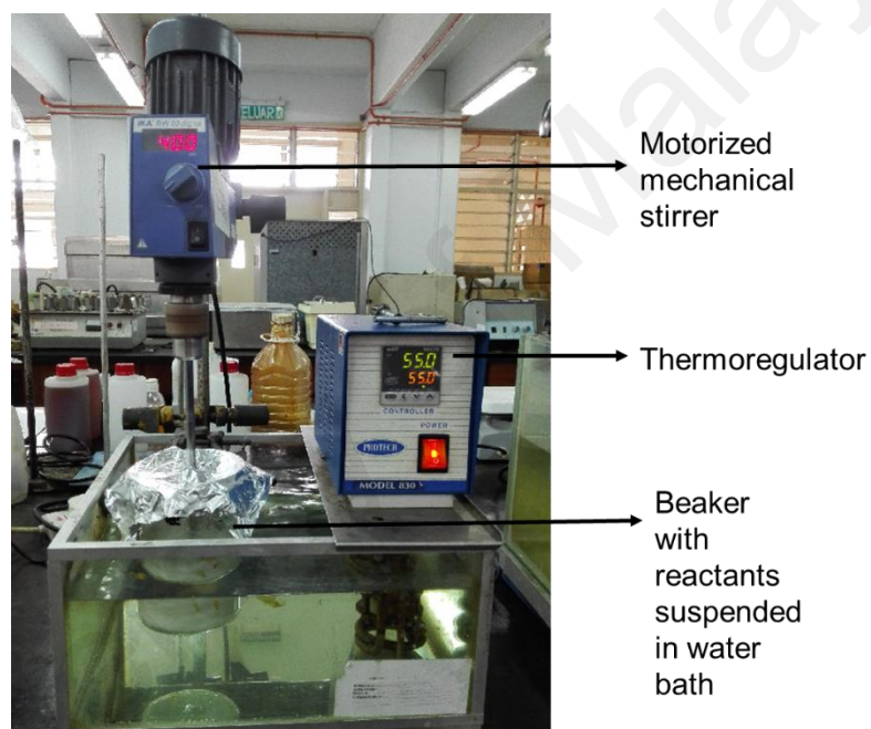
Fig. 3.3: Experimental set up of microencapsulation process
