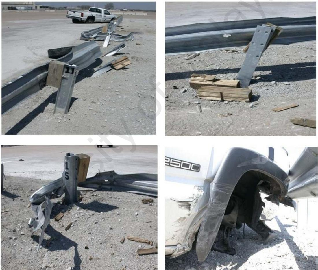
Figure 2-16. Summary of the test results for the guardrail systems subjected to the full-scale crash tests (Polivka et al., 2006b)
