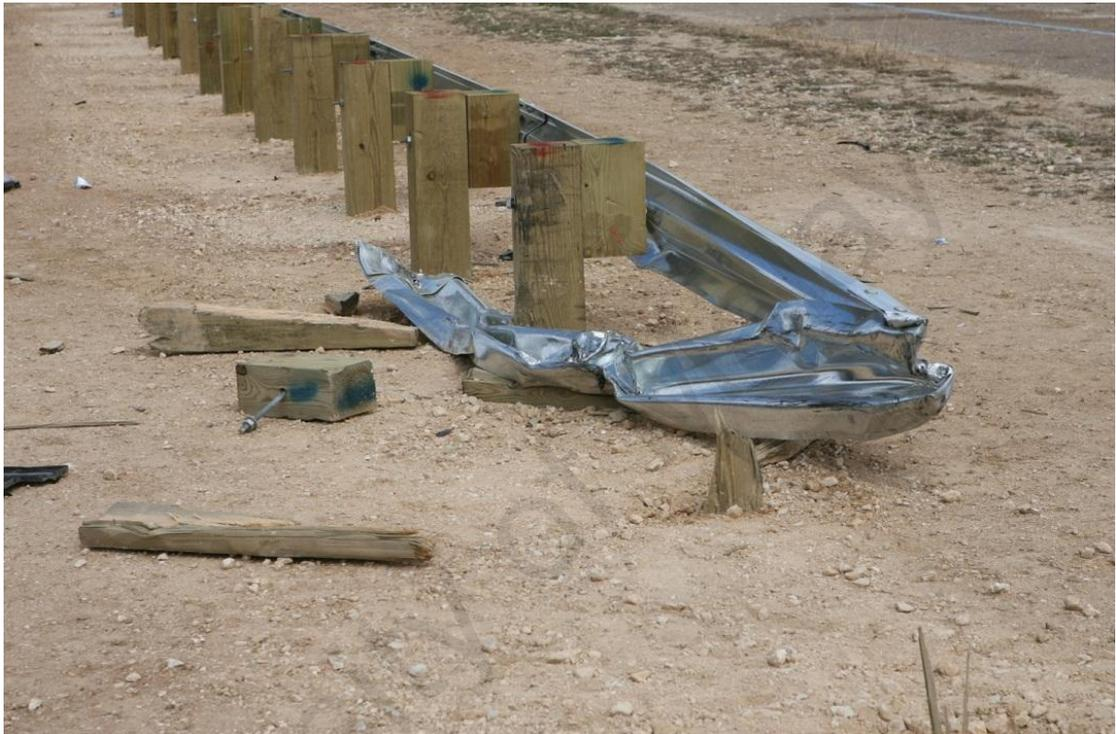
Figure 2-17. Rail rupture in the G4(2W) guardrail system (Bullard et al., 2010a)
