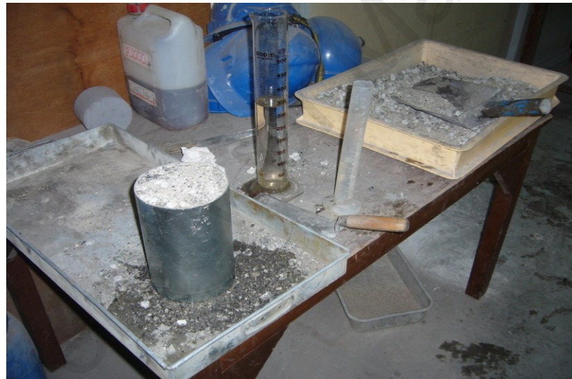
Figure 3.5: Particle packing test set-up
