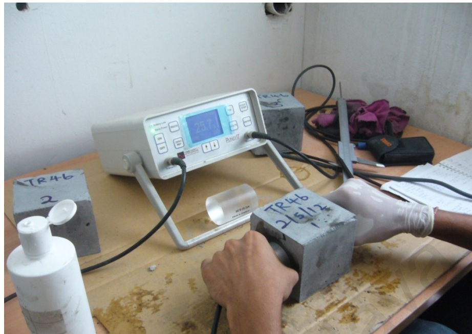
Figure 3.18: UPV test for concrete specimen
