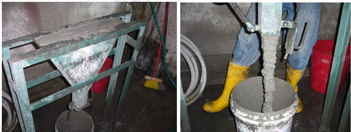
Figure 3.10: V-funnel test set-up
