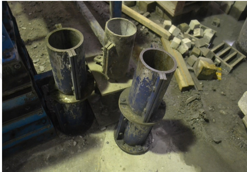
Figure 3.20: Splitting tensile strength molds (200 mm × 100 mm diameter)
