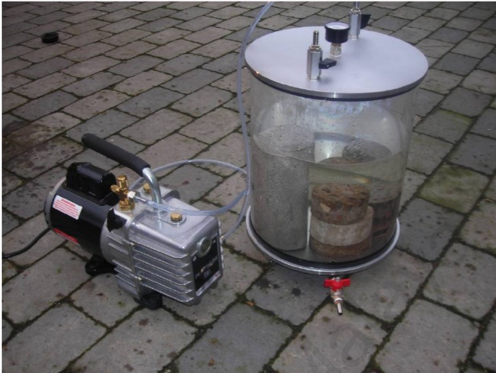
Figure 3.22: Rapid chloride penetration test vacuum pump and dessicator (Adapted from PROOVE'it Instruction and Maintenance Manual)
