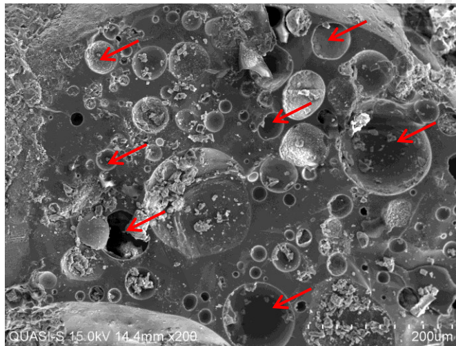
Figure 5.32: Presence of substantial amount of voids on POC fine aggregates in mortar (as indicated by the red arrows)
