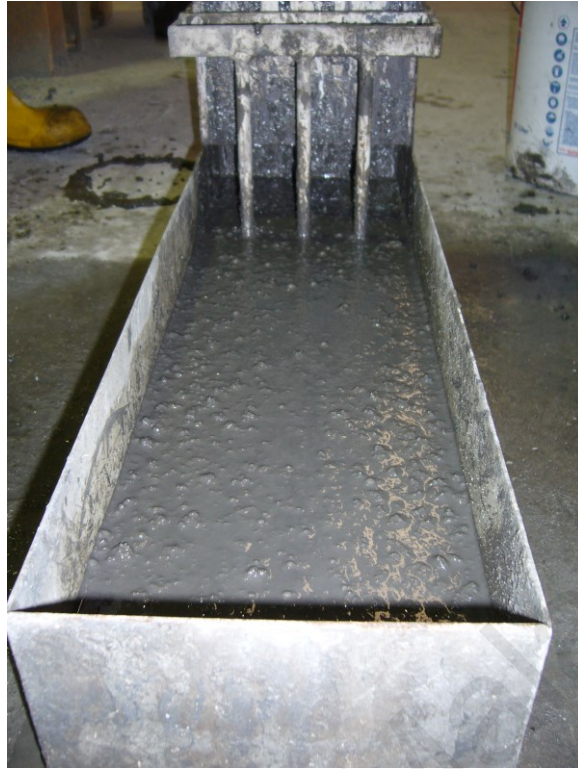
Figure 3.12: L-box test set-up
