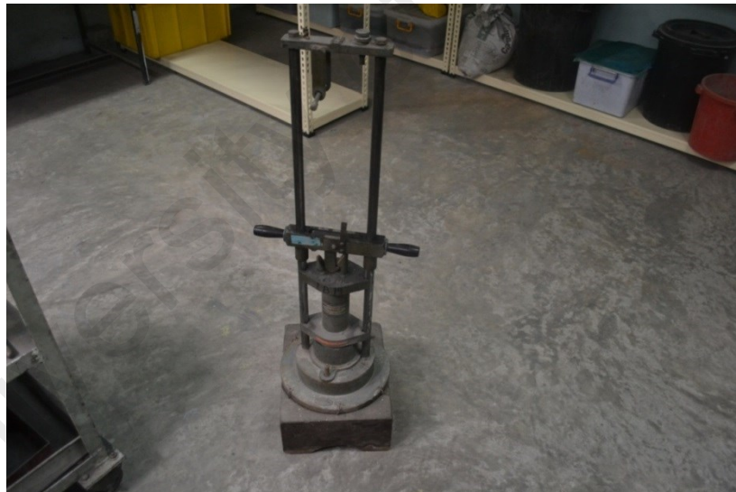
Figure 3.1: Aggregate impact value test setup
