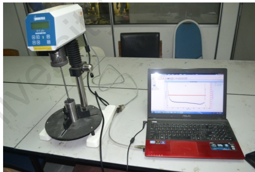
Figure 3.14: A Brookfield rheometer with Rheo3000 software
