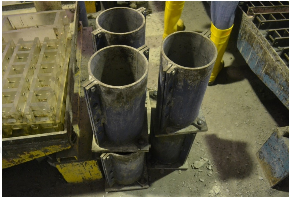
Figure 3.21: Modulus of elasticity molds (300mm × 200mm diameter)
