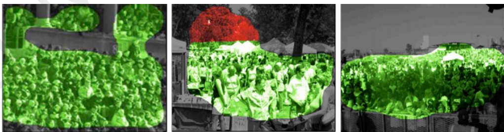
Figure 2.3: Sample results of dense crowd segmentation where regions containing crowd are segmented using method as proposed by Arandjelovic (2008). The true positives are highlighted in green whereas the false positives are represented by the red areas. Best viewed in color. ((Arandjelovic, 2008))
