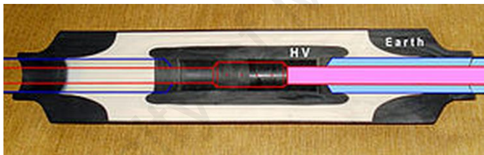
Figure 2.1: Bi-manchet at the XLPE cable joint
