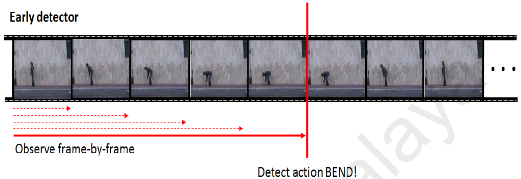
Figure 1.1: Traditional detector versus early detector. The traditional detector detect an action after fully observing the video, whereas the early detector detects an action by observing the video frame-by-frame, such that it able to detect an action before its completion.
