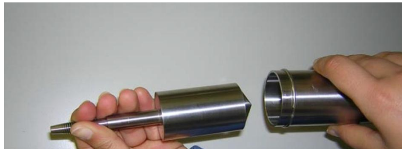
Figure 3.2 Cup and geometry used for measuring rheology properties of ice creams.
