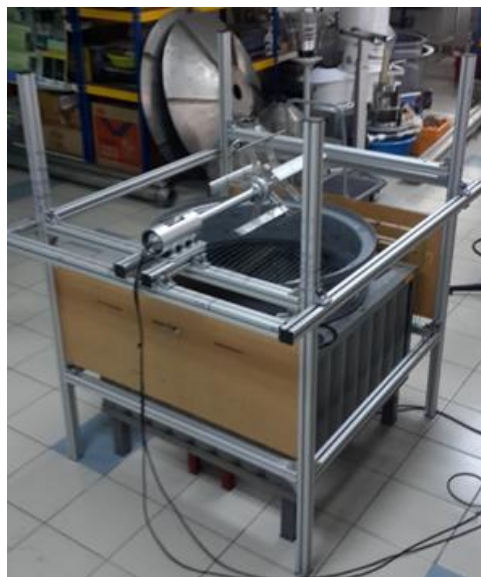
Figure 3.14 Test rig, consisting of cooling tower model, wind turbine, dynamometer and supporting frame.
