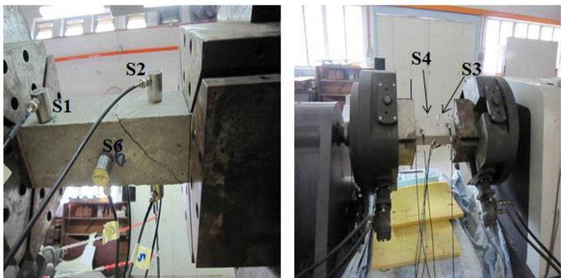
Figure 3.2: Torsion tests on concrete beams and AE sensor placement
