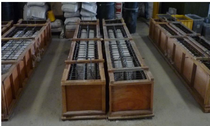
Figure 3.5: Molds, polystyrene and reinforcement cages overview
