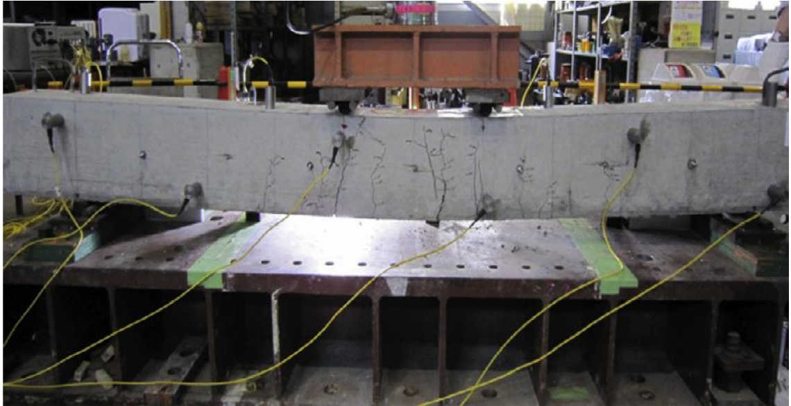
Figure 4.51: Failure pattern of PFRC specimen at ultimate load
