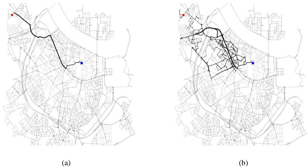
Figure 1.1: Comparison between proposed paths by (a) static and (b) dynamic algorithms for the same OD pair
