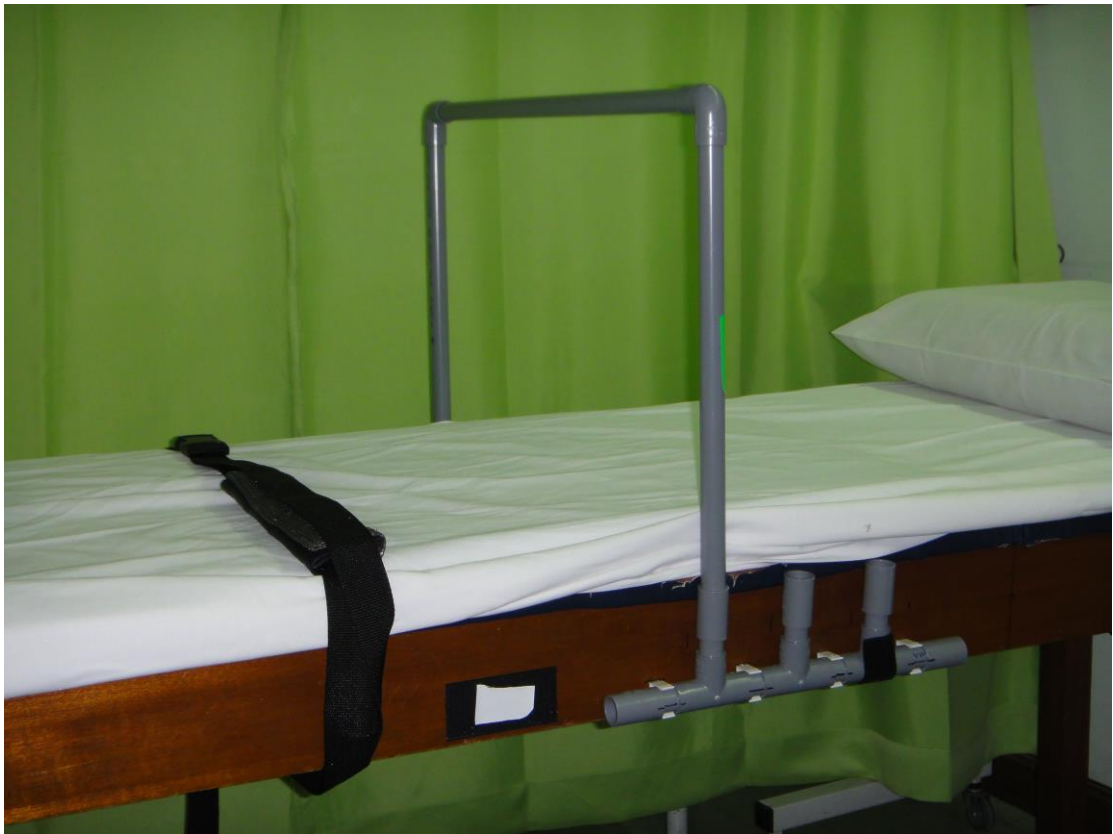
Figure 4.6. Apparatus used to aid active knee extension (AKE) test constructed from polyvinyl chloride (PVC) tubes.
