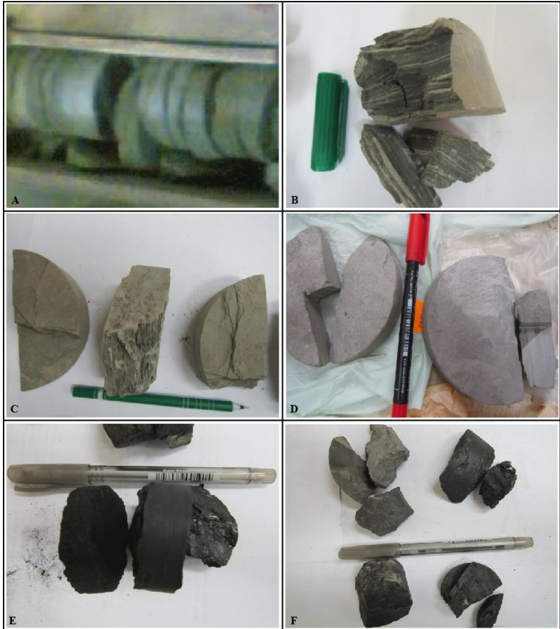
Fig.3.1.1. (A) Shale and sandstone core samples stored in core-box of BAPEX; (B) and (C) Shale core samples; (D) Sandstone core samples; (E) Coal core samples of the Dighipara Basin; (F) Coal core samples with organic-rich mudstone (top left at F) sample of the Barapukuria Basin.
