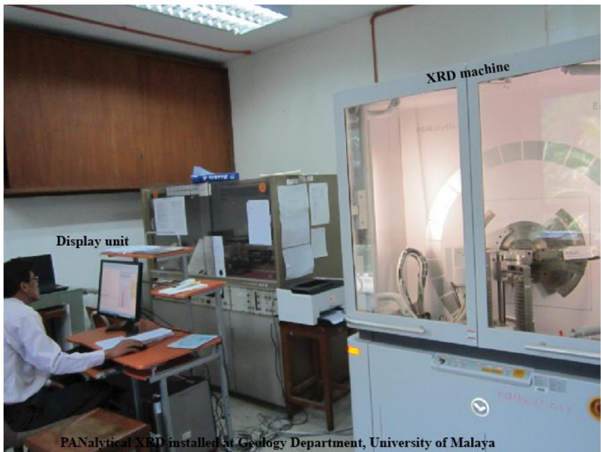
Fig.3.2.13. A PANalytical X-ray Diffraction (XRD) machine working at the Geology Department of the University of Malaya.
