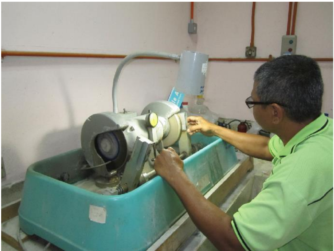
Fig.3.2.10. Thin section preparation in progress operated at the Geology Department, University of Malaya.
