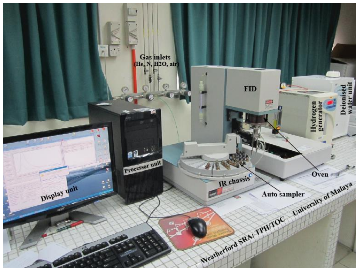
Fig.3.2.1. A Weatherford Source Rock Analyzer (SRA:TPH/TOC) installed at the petroleum geochemistry laboratory of the Geology Department, University of Malaya.
