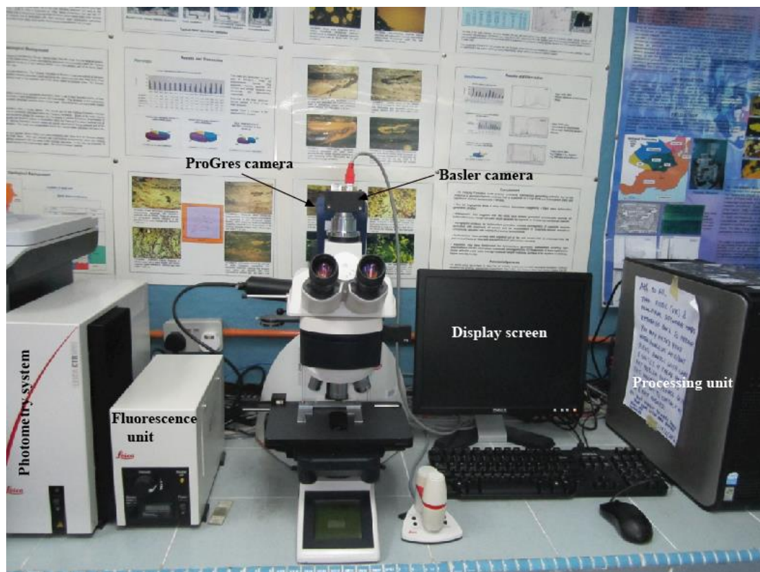
Fig.3.2.8. A LEICA DM6000M microscope and LEICA CTR6000 photometry system equipped with fluorescence illuminators used at the Geology Department of the University of Malaya.
