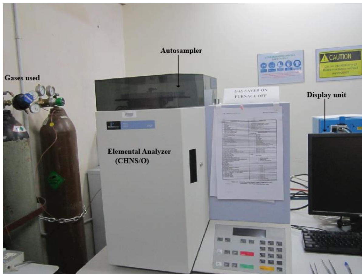
Fig.3.2.2. A Perkin Elmer 2400 elemental analyzer (CHNS/O) operated at the Chemistry Department of the University of Malaya.
