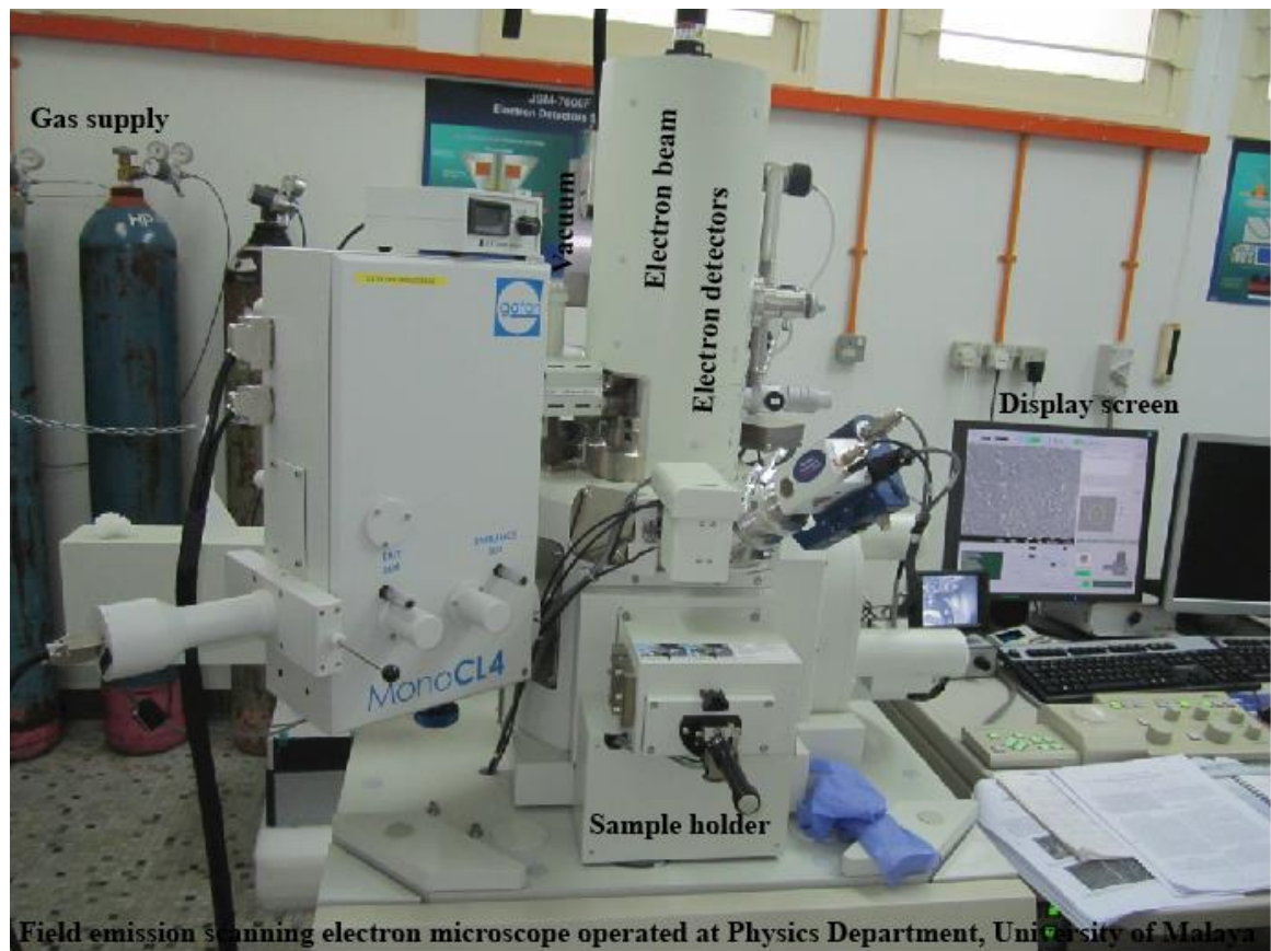
Fig.3.2.12. A JEOL JSM-7600F field emission scanning electron microscope (FESEM) operated at the Physics Department of the University of Malaya.
