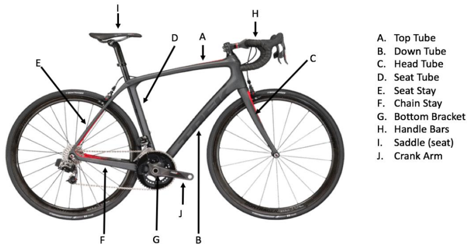
Figure 1. Diagram with labels of key components of the bicycle.
