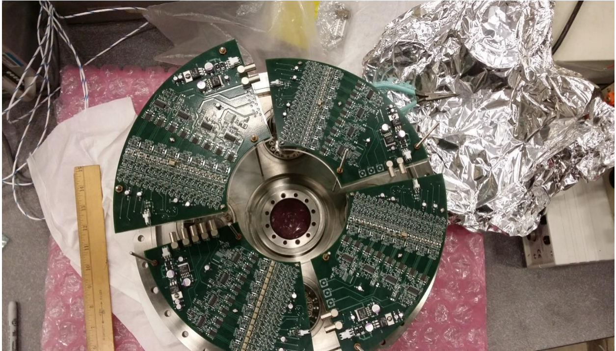
Figure 5: The electronic boards arranged above the main flange. The SiPM detectors plug in on the other side.
