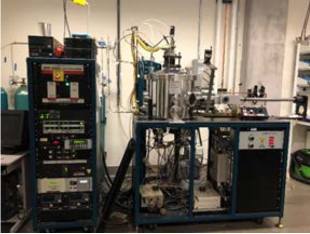
Figure 4: Image of the AJA International ATC 2000 Sputtering System.
