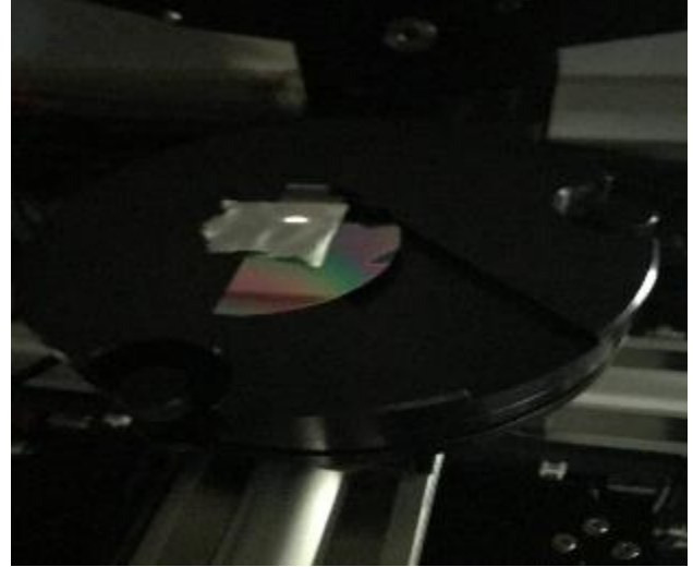
Figure 12: Sample 1 as deposited being analyzed with the ellipsometer. In this image the paper helps align the beam with the correct portion of the sample between the desired scratches.
