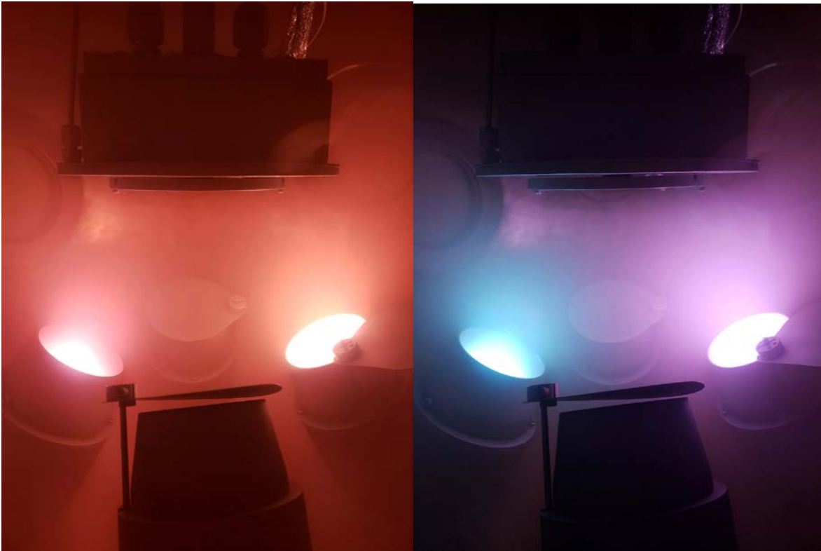
Figure 34: (Left) Sputtering targets before nitrogen was flowed into the chamber; (Right) sputtering targets after Nitrogen was flowed into the chamber. It is easier to distinguish between the two metal targets in the image on the right.
