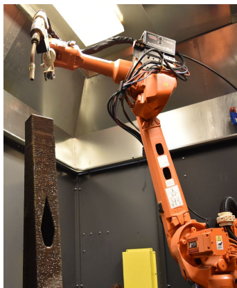
Figure 1. Wolf robotic arm used for additive manufacturing. A MIG welding torch is mounted to the end of the actuator.
