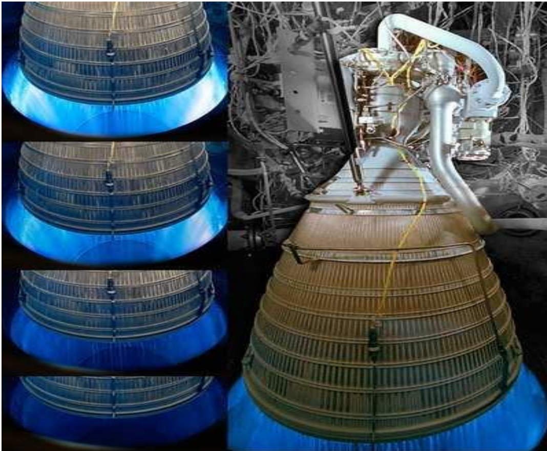
Figure 10. RL10 CECE rocket engine throttling from 10:1 [33]
