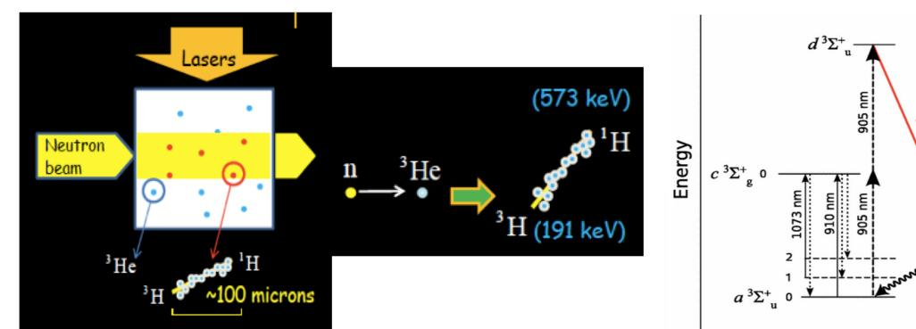
These tracers only track the normal fluid phase (> 1K) and do not perturb the flow.
