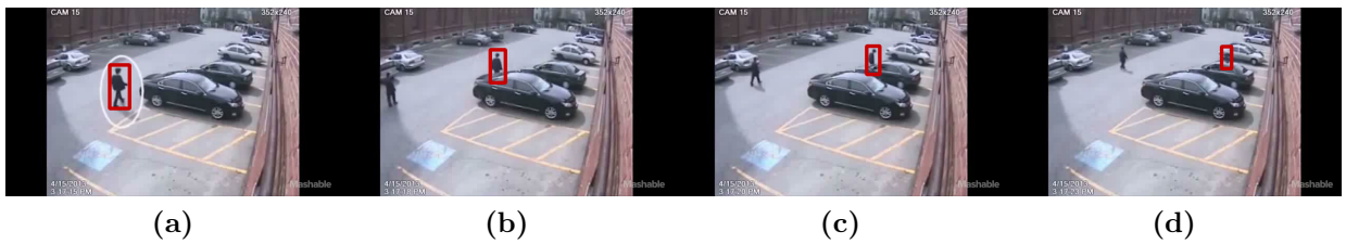
Figure 3.19: Despite the low resolution and partial occlusion, SiamFC tracks the subject into the car.
