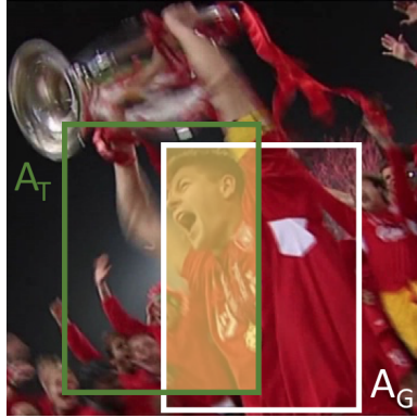
Figure 1.12: Trackers attempt to place an estimated bounding box A_T with as large an overlap (yellow) as possible with the ground truth A_G . (Background image from [8])
