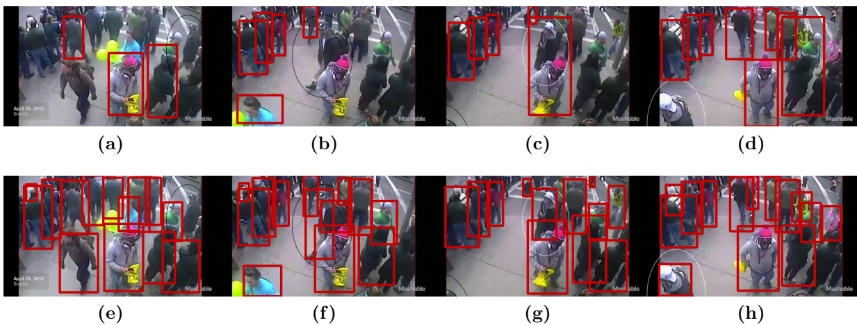
Figure 3.9: In crowds, the tiny network misses many partially occluded or rotated individuals. (tiny a-d, normal e-h)
