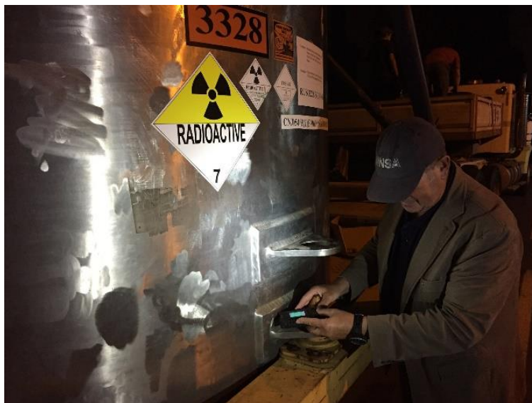
Figure 3.2. Gamma dose rate monitor of cask containing the GHARR-1 HEU core
