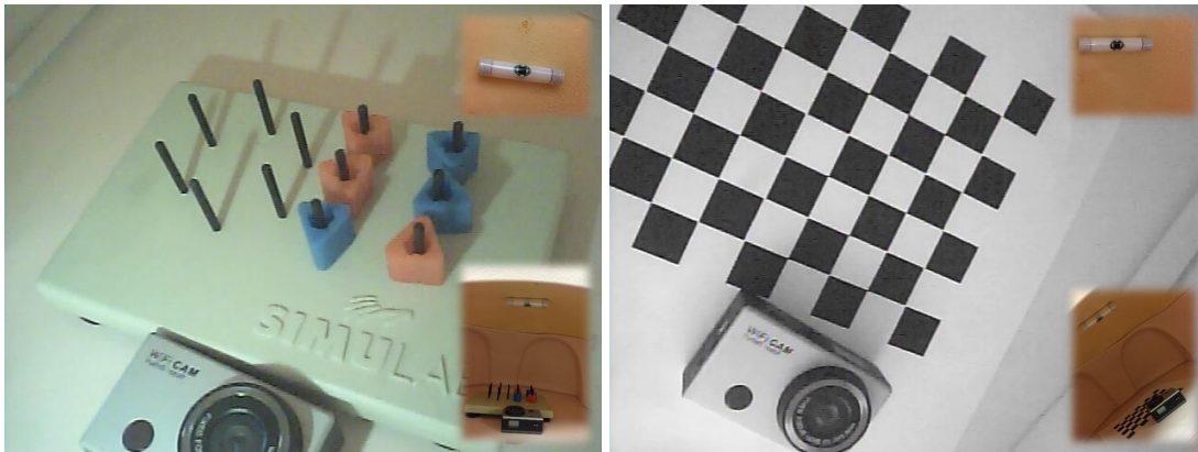
Figure 3.7: Wireless imaging performance test. A picture of the anchored robotic surgical camera taken by a wifi camera is shown in a top-right insets.
