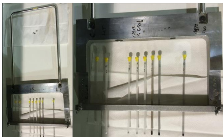
Figure 10: NMR tubes loaded with radioactive powders mounted on the NOMAD sample shifter tray for room-temperature neutron scattering measurements
