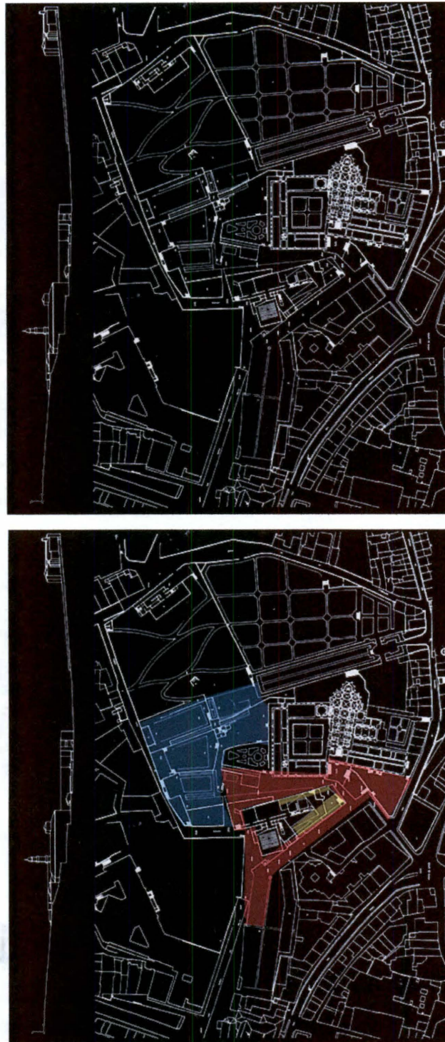
Figure 46 (A &B). The Centro Gallego de Art Contemporaneo, Santiago de Compostela, Spain by Alvaro Siza. The boundaries of the site are indicated in red, the garden in blue and the transition zones in yellow.
