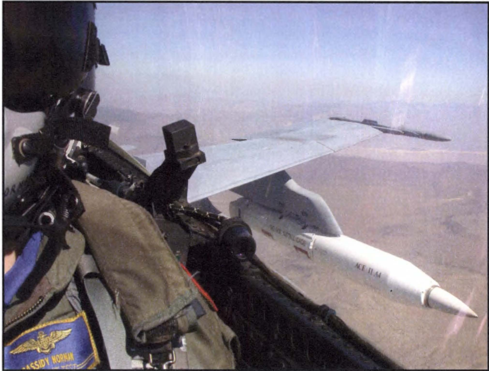
Figure 4: ACE pod used for captive AMRAAM testing
