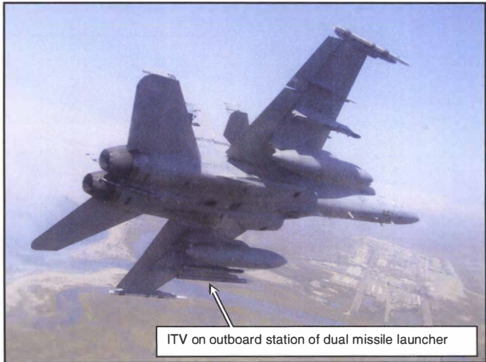
Figure 5: ITV pod used for captive AMRAAM testing
