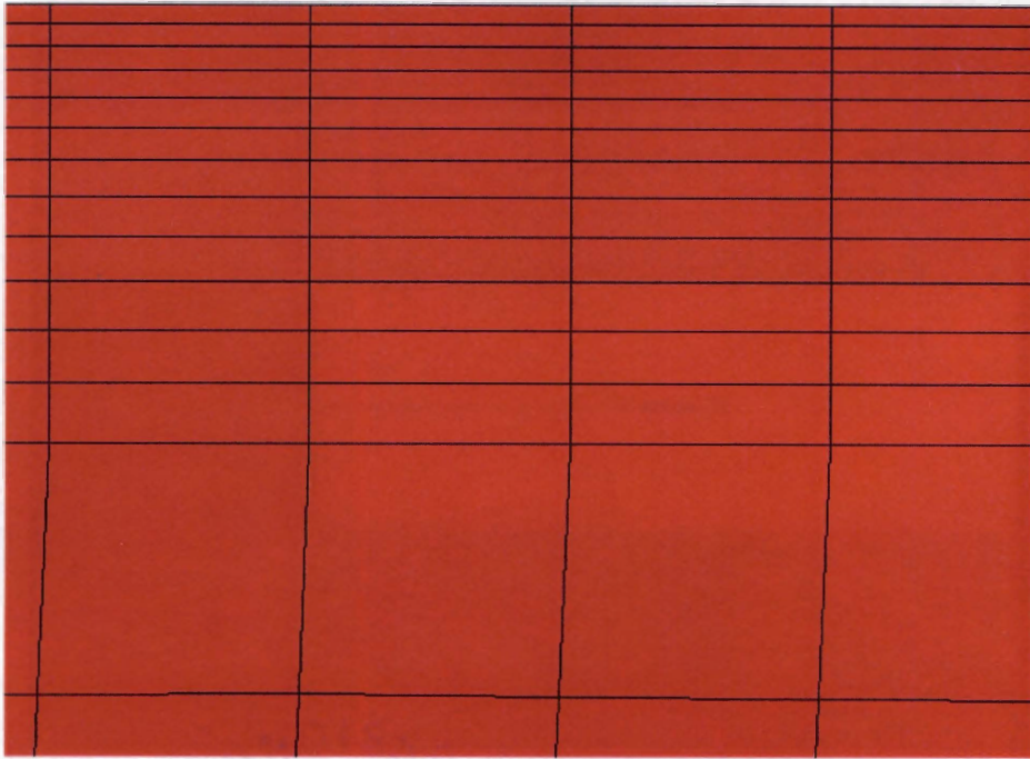
Figure D.4: FLUID141 FEM Detail Near Wall
