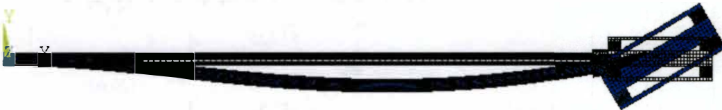
Figure 61: Sting + Nut + Balance and Calibration Device Mesh for Constrained Condition Plot of 2 nd Mode Shape (distorted)
