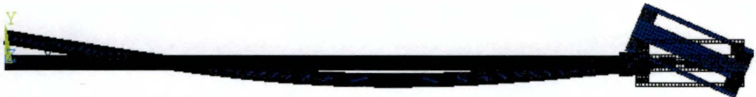
Figure 67: 2 nd Mode Shape for Unconstrained Condition (distorted)
