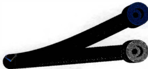
Figure 57: Sting + Nut Mesh for Constrained Condition – Plot of 1 st Mode Shape (distorted)
