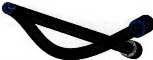
Figure 58: Sting + Nut Mesh for Constrained Condition – Plot of 2 nd Mode Shape (distorted)
