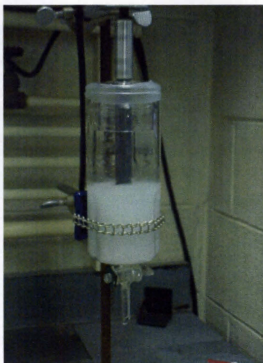
Figure 2. Thick Emulsion Formed During Solvent Extraction
