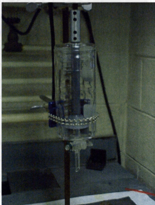
Figure 1. Reaction Apparatus Used For Solvent Extraction Experiments
