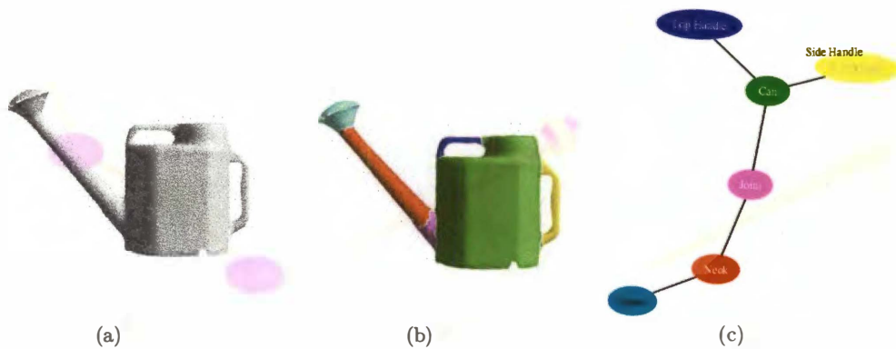
Figure 7.12: Watering can decomposition. Minima Rule Algorithm results for a watering can. This mesh is a reconstruction from the Polhemus FastSCAN System. The mesh consists of 8,086 vertices and 15,843 triangles while the decomposition consists of 6 parts. (a) Rendering of original mesh. (b) Decomposition of mesh into parts. (c) Adjacency graph with user-specified labels.
