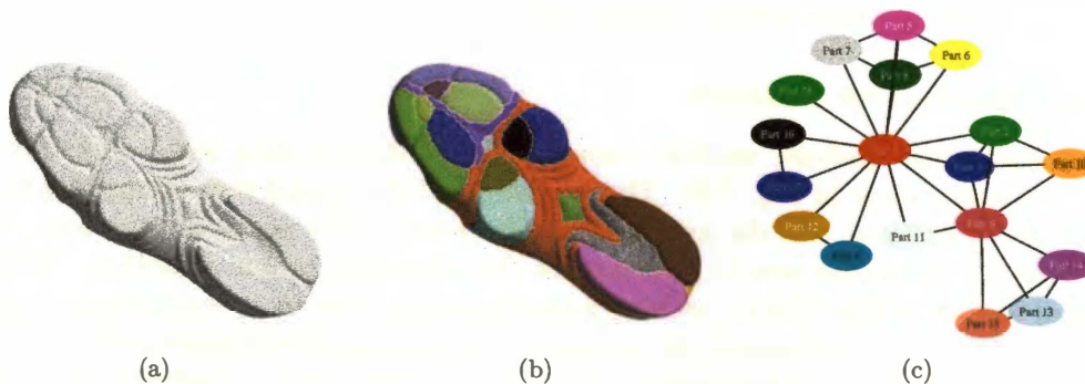
Figure 7.22: Shoe sole decomposition. Minima Rule Algorithm results for a shoe sole. The mesh is a reconstruction from the 3D Digital Corporation. The mesh consists of 58,108 vertices and 115,750 triangles while the decomposition consists of 18 parts. (a) Rendering of original mesh. (b) Decomposition of mesh into parts. (c) Adjacency graph with arbitrary labels.
