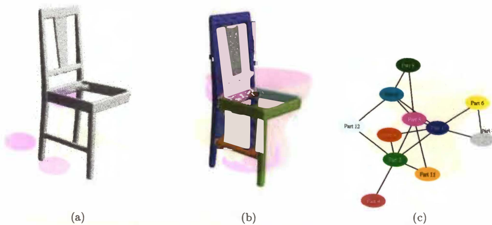
Figure 7.13: Three-legged chair decomposition. Minima Rule Algorithm results for a three-legged chair. This mesh is a reconstruction from the Polhemus FastSCAN System. The mesh consists of 26,766 vertices and 53,462 triangles while the decomposition consists of 11 parts. (a) Rendering of original mesh. (b) Decomposition of mesh into parts. (c) Adjacency graph with arbitrary labels.
