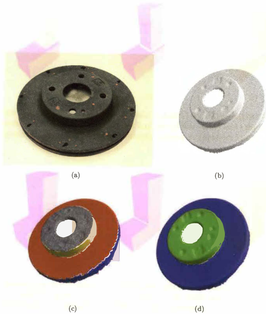
Figure 7.40: Comparison of segmentation algorithms for automotive disc brake. A comparison of segmentation results for a simple scene consisting of a box resting on a floor. (a) Photograph of actual disc brake. (b) Rendering of reconstructed triangle mesh. (c) Segmentation results for Mangan and Whitaker's algorithm with four regions. (d) Segmentation results for the proposed algorithm with two regions—the inner and outer disc.
