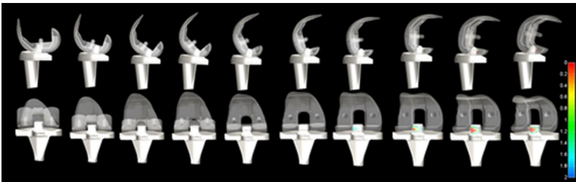
Figure 5-11: Example of cam-post contact for a patient in the Zimmer PS FB TKA group
