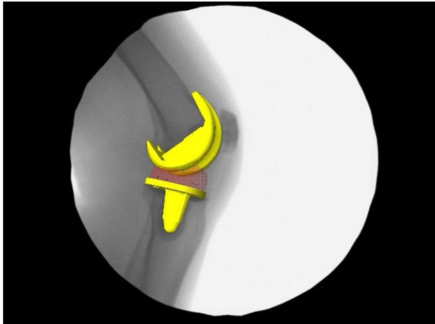
Figure 4-5: Fluoroscopy image with femoral and tibia CAD model of Sigma PS RP TKA and four visible bead silhouettes that allow for proper positioning of PE bearing when silhouettes match.
