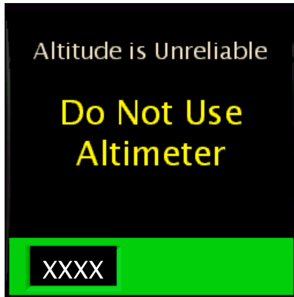
Figure 32. Display Fault Indication Symbology
