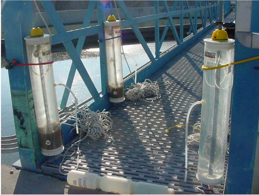
Figure 4: DSS samples taken in Kemmerer samplers during settling
